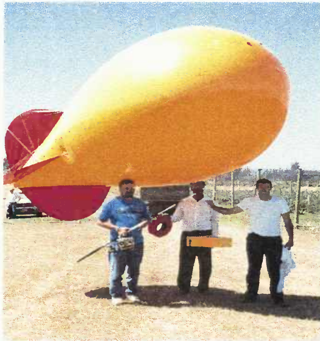
Figure 3.1 The helium filled blimp and camera mounted platform
