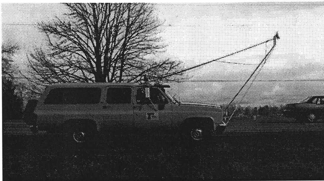
Figure 3.2 Survey Vehicle and Camera Mounting Devices.
