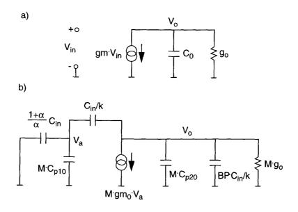
Figure 3.9: Small-signal model of a single-pole amplifier in a) stand-alone configuration. b) feedback configuration.
