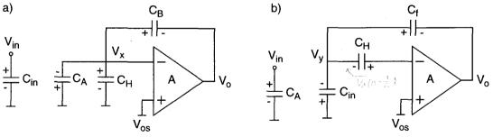
Figure D.2: Predictive Nagaraj integrator and timing diagram. a) Configuration during phase #1, for  $t = n - 1/2 - \varepsilon$  ( $\varepsilon \ll 1$ ). b) Configuration during phase #2, for  $t = n - \varepsilon$ .
