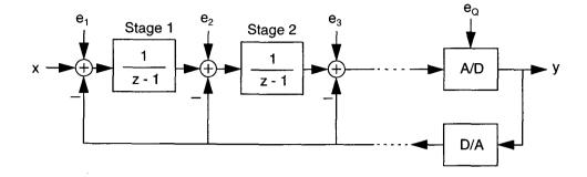
Figure 2.4: Simplified block diagram of an idealized  $\Delta\Sigma$  modulator of arbitrary order.
