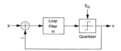
Figure 2.1: Simplified block diagram of a delta-sigma modulator.
