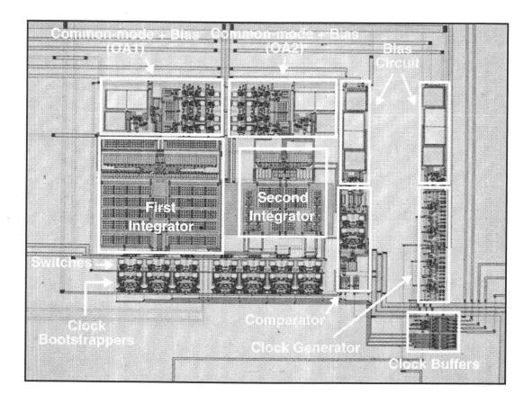
Figure 4.11: Chip microphotograph.
