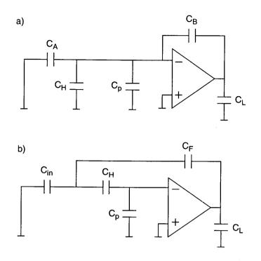
Figure 5.9: Circuit configuration of a predictive Nagaraj integrator in the a) prediction phase and the b) integration phase.
