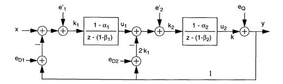
Figure 3.1: Block diagram of a 2nd-order delta-sigma modulator with indication of various noise sources.
