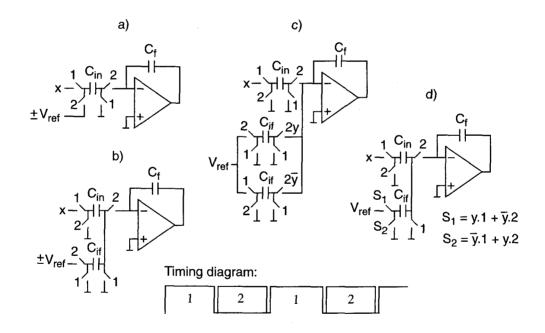
Figure 3.6: Switched-capacitor, single-ended implementation of the first integrator with a) double reference voltage -- single input branch, b) double reference voltage -- two input branches, c) single reference voltage -- two input branches, and d) single reference voltage -- two input branches.
