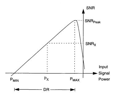
Figure 2.3: Performance metrics used in connection with delta-sigma modulators.
