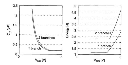
Figure 3.8: a) Minimum size of the input capacitor when one and two SC branches are utilized in the input stage, as a function of  $V_{DD}$ , and b) Power dissipation per cycle (energy) when one and two SC branches are utilized in the input stage, as a function of  $V_{DD}$ .
