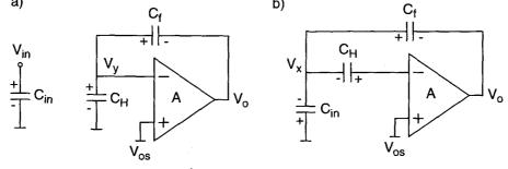
Figure D.1: Nagaraj integrator and timing diagram. a) Configuration during phase #1, for  $t = n - 1/2 - \varepsilon$  ( $\varepsilon \ll 1$ ). b) Configuration during phase #2, for  $t = n - \varepsilon$ .
