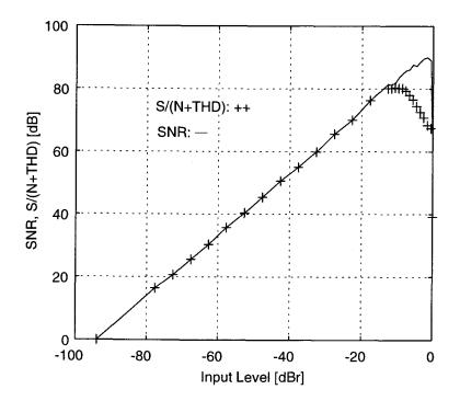
Figure 4.12: Measured SNR and S/(N + THD) as functions of the input signal level.
