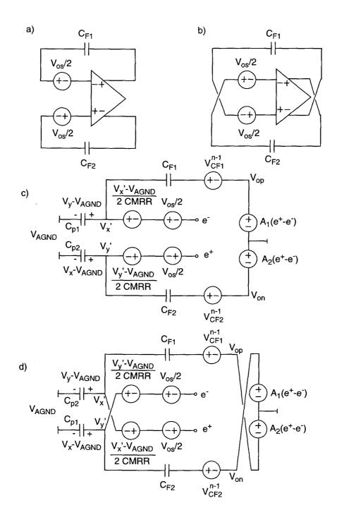
Figure B.7: Possible configurations when chopper stabilization is used. a) Configuration #1. b) Configuration #2. c) Model to update node voltages in configuration #1. d) Model to update node voltages in configuration #2.
