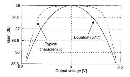
Figure 5.4: Op-amp nonlinear dc gain characteristic as given by (5.17), for  $A_0 = 38 \,\mathrm{dB}$ ,  $\gamma_1 = 0.01 \,\mathrm{V}^{-1}$  and  $\gamma_2 = 1.2 \,\mathrm{V}^{-2}$  (solid line). Also shown is a typical gain characteristic of an amplifier (dashed line).
