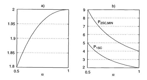
Figure 3.7: a) Ratio between  $P_{2SC,MIN}$  and  $P_{ISC}$ . b)  $P_{2SC,MIN}$  and  $P_{ISC}$  normalized to  $2 \cdot kT \cdot DR/OSR$ .
