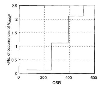
Figure 3.5: Average number (simulated) of occurrences of  $V_{MAX}$ , per period of the (sinusoidal) input signal, as a function of the oversampling ratio.
