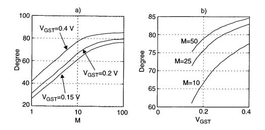
Figure 4.6: Phase margin as a function of a) multiplicity M, parameter is gate overdrive voltage, and b) gate overdrive voltage  $V_{GST}$ , parameter is multiplicity.
