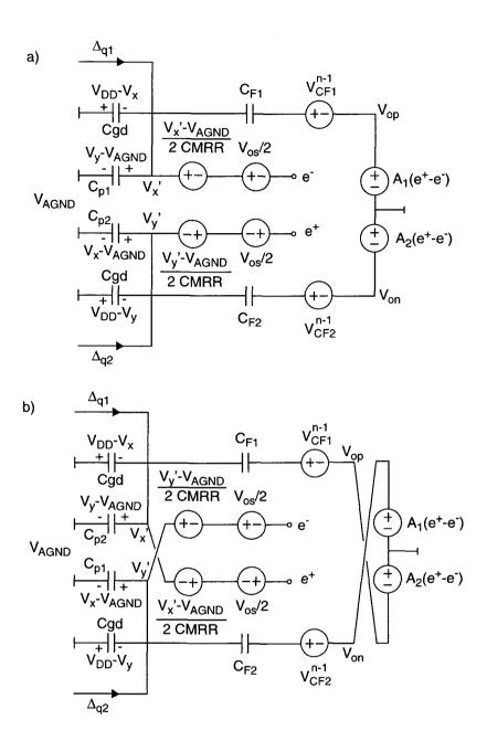
Figure B.9: Model for clock charge injection in the end of phase #2. a) Configuration #1. b) Configuration #2.
