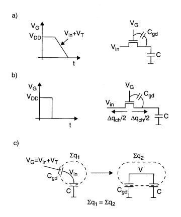
Figure B.4: Modeling of the clock charge injection. a) Slow-switching mode. b) Fast-switching mode. c) Charge conservation principle.
