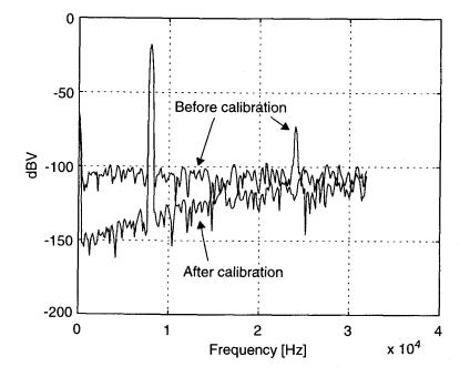
Figure 3.18: Simulated spectrum of the output of a 2nd-order delta-sigma modulator employing 4-bit quantization, with and without calibration of the D/A converter. The sampling frequency was 2.048 MHz, the capacitor mismatch in the uncalibrated DAC was 0.5%, and the number of samples 16,384. The uncalibrated DAC had a differential nonlinearity of 85 16-bit LSBs, and the calibrated DAC 0.52 16-bit LSBs.
