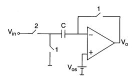
Figure 5.1: SC voltage comparator employing correlated double sampling for offset compensation.
