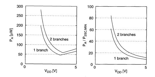
Figure 3.11: a) Amplifier (fully-differential folded-cascode) static power dissipation. b) Ratio between the amplifier static power dissipation and the minimum dynamic power dissipation in the sampling network.
