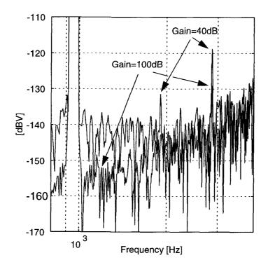
Figure 3.4: Effect of the nominal dc gain on distortion. The input signal was a - 17.4 dBV (-10 dBr),  $3/\pi$  kHz sinewave, and the sampling frequency 2 MHz.
