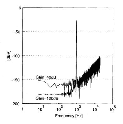
Figure 3.3: Quantization noise leakage due to op-amp finite dc gain. The input signal was a -22.4 dBV (-15 dBr),  $3/\pi$ kHz sinewave, and the sampling frequency 2 MHz.
