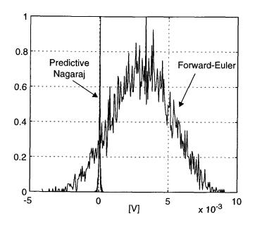
Figure 5.7: Histograms of the virtual ground signal for a forward-Euler integrator and a predictive Nagaraj integrator.
