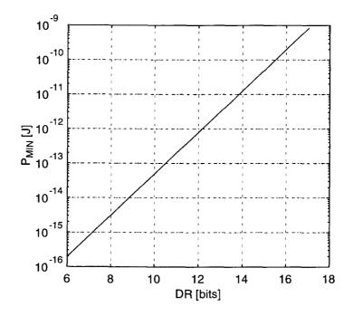
Figure 2.7: Minimum energy consumption (power per bandwidth) as a function of the dynamic range.
