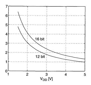
Figure 3.12: Ratio between the minimum current to obtain the required closedloop bandwidth, and the minimum current required for slewing, for DR = 12 bits and DR = 16 bits.
