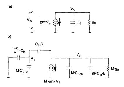
Figure A.1: Small-signal model of a single-pole amplifier a) in a stand-alone configuration and b) in a feedback configuration.
