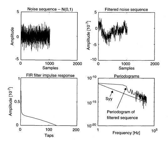
Figure B.3: Generation of a noise time signal for simulation of flicker noise, from a filtered pseudo-random white noise sequence.
