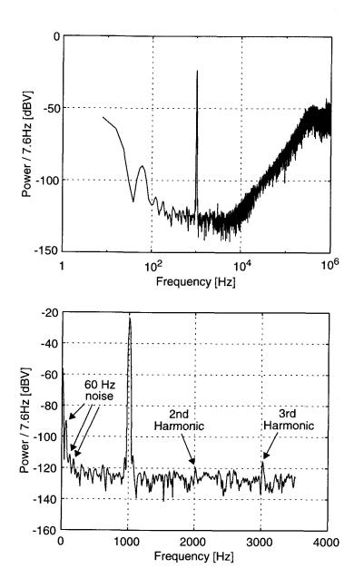
Figure 4.13: Measured output spectrum for a -12.6 dBr, 1 kHz sinewave input. Noise power = -99.21 dBV, Signal power = -20 dBV.
