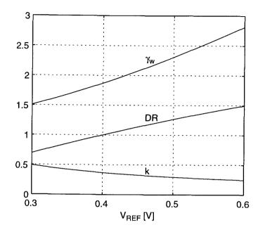
Figure 3.16: Dynamic range as a function of the reference voltage, normalized to the value obtained when  $V_{REF} = 0.4$  V. Also shown are the excess noise and gain factors.
