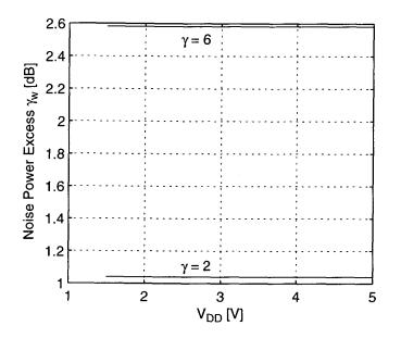
Figure 3.14: Thermal noise excess factor at the input, due to amplifier noise.
