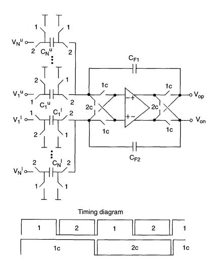
Figure B.5: Circuit diagram of a generalized fully-differential switched-capacitor integrator with chopper stabilization.
