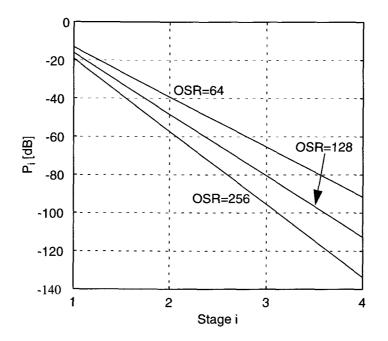
Figure 2.5: Attenuation of the noise power generated at the input of stage *i*.
