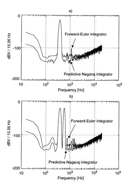
Figure 5.5: Output spectra of a 2nd-order delta-sigma modulator when the input stage is a forward-Euler SC integrator and when the input stage is a predictive Nagaraj integrator. a) The input signal is a 400 Hz sinusoid with power -10.5 dBV. b) The input signal is a 2-tone, 400 Hz and 600 Hz, signal, each tone with power -16 dBV. The sampling frequency was 2 MHz in both cases, and the assumed op-amp dc offset voltage was 3 mV.
