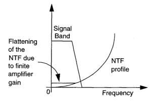
Figure 3.2: Effect of the amplifier finite dc gain on the noise transfer function.
