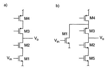
Figure 3.10: Simplified single-ended implementation of a a) telescopic cascode amplifier. b) folded-cascode amplifier.
