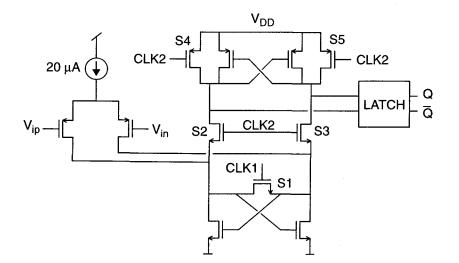
Figure 4.10: Comparator circuit.
