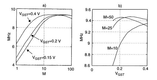
Figure 4.5: Unity-gain bandwidth as a function of a) multiplicity M, parameter is gate overdrive voltage, and b) gate overdrive voltage  $V_{GST}$ , parameter is multiplicity.
