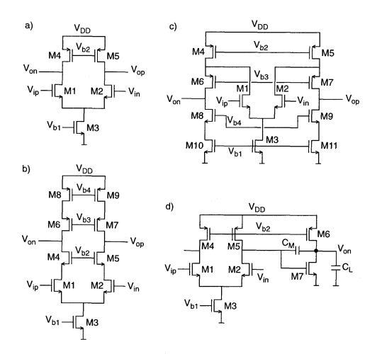
Figure 3.17: Four popular amplifier topologies: a) differential pair, b) telescopic cascode amplifier, c) folded-cascode amplifier, and d) two-stage Miller amplifier.
