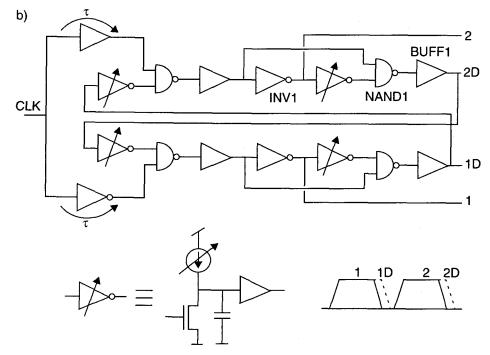
Figure 4.1: a) Fully differential switched-capacitor implementation of the 2ndorder delta-sigma modulator. b) Four-phase clock generator and timing diagram.
