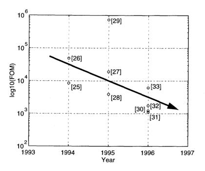
Figure 2.8: Trend for efficiency of utilization of energy. A large *FOM* means less efficiency.
