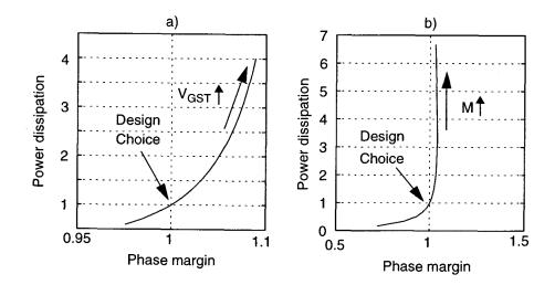
Figure 4.7: Normalized power dissipation ( $V_{DD} = 1.8$  V) as a function of the normalized phase margin: a) for  $V_{GST} = 0.15 \dots 0.4$  V. b) for M = 1 to 200.
