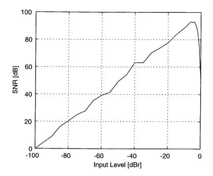
Figure 4.2: Simulated *SNR* as a function of the input signal level power, for a 1 kHz frequency input sinewave.
