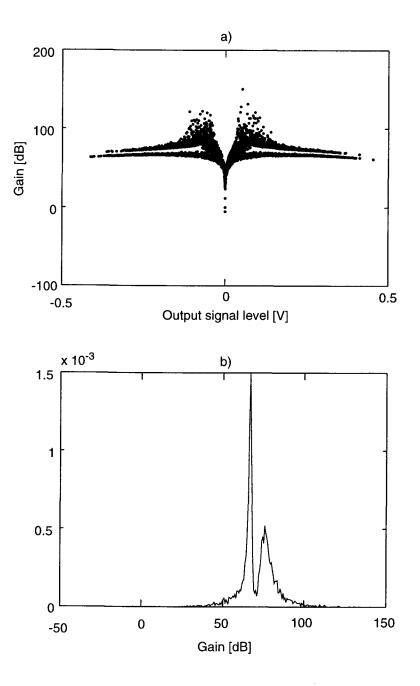
Figure 5.6: Equivalent dc gain of the amplifier. a) As a function of the output signal level. b) Histogram of 5000 samples.
