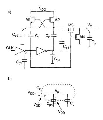
Figure C.1: Voltage doubler. a) Circuit diagram, with indication of the parasitic capacitances. b) Right-hand side circuit configuration when CLK is "high."
