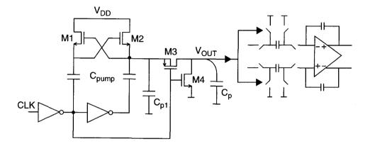
Figure 4.3: Clock bootstrapping stage.
