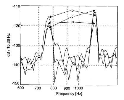
Figure 5.8: Magnified output spectrum of a 2nd-order delta-sigma modulator (showing signal harmonics) when the input stage is a predictive Nagaraj integrator. Curve <u>a</u> corresponds to utilizing a nominal gain of 38 dB in both prediction and integration phases. Curve <u>b</u> corresponds to utilizing a 20% lower gain in the prediction phase, and curve <u>c</u> corresponds to utilizing a 20% lower gain in the integration phase.
