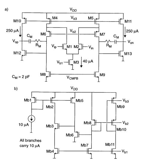
Figure 4.8: a) Complete circuit diagram of the first stage amplifier. b) Bias circuit.
