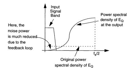
Figure 2.2: The concept of noise shaping.
