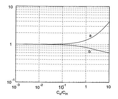
Figure 3.15: Amplifier load capacitance with  $C_o$ , normalized to that without  $C_o$ , (a), and input capacitor size with  $C_o$ , normalized to that without  $C_o$ , (b), as a function of the ratio  $C_o/C_{in}$ .
