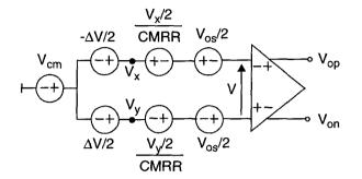
Figure B.2: Modeling of the op-amp dc offset voltage and common-mode rejection ratio (*CMRR*).
