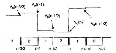
Figure 5.3: Typical waveform for the output voltage of a SC integrator in a deltasigma modulator.
