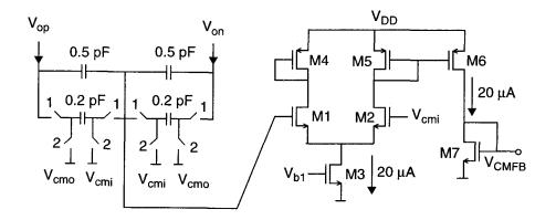
Figure 4.9: Common-mode circuit.
