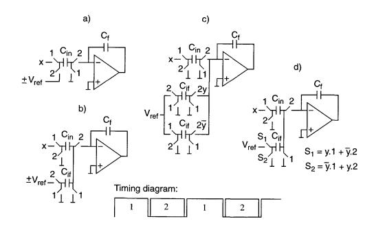
Figure 3.19: Switched-capacitor, single-ended implementation of the first integrator with a) double reference voltage -- single input branch, b) double reference voltage -- two input branches, c) single reference voltage -- three input branches, and d) single reference voltage -- two input branches.
