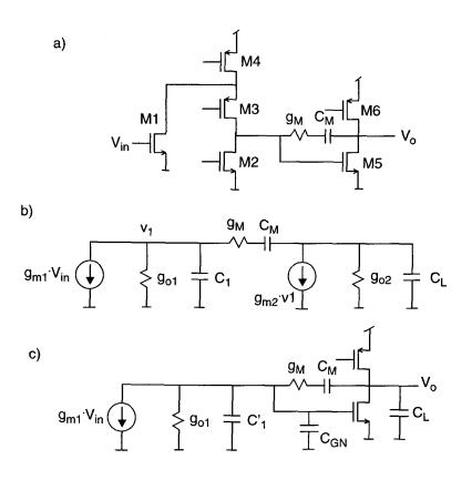
Figure 4.4: Two-stage amplifier with Miller frequency compensation. a) Simplified single-ended circuit. b) Simplified linear model. c) Detail of output stage.
