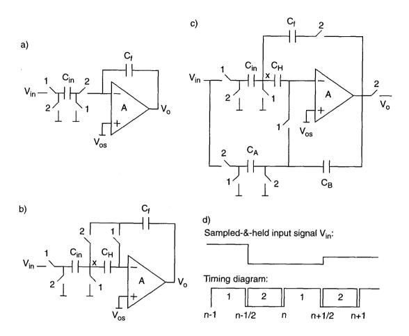
Figure 5.2: Three SC integrator topologies: a) Regular forward-Euler integrator.b) Offset- and gain-compensated Nagaraj integrator. c) Predictive Nagaraj integrator. d) Timing diagram and sampled-and-held input signal of the predictive Nagaraj integrator.
