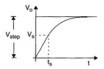
Figure B.10: Transient response of an amplifier to a step voltage, showing slewing behavior  $(t < t_s)$  and linear settling behavior  $t > t_s$ .
