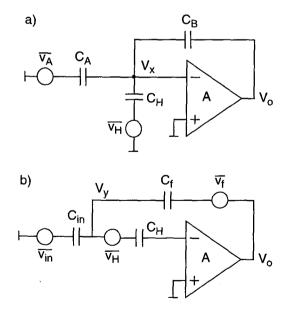
Figure 5.11: AC model of a predictive Nagaraj integrator showing the kT/C noise sources during a) prediction phase and b) integration phase.
