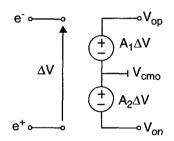
Figure B.1: Basic model of a fully-differential op-amp with finite dc gain.
