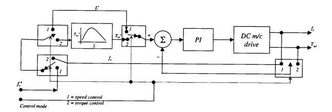
Figure 4.2 DC machine based wind-turbine model controller.
