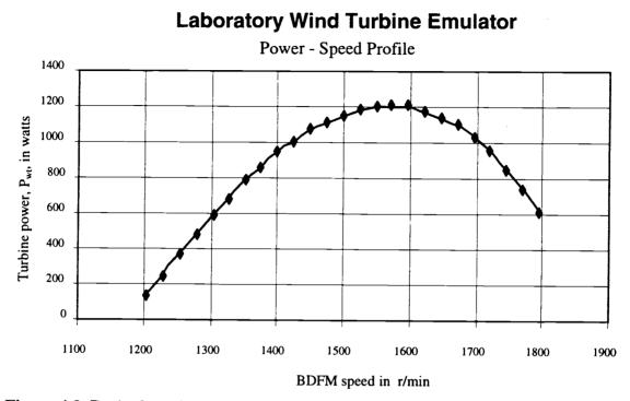
Figure 4.3 Desired mechanical power output of the laboratory wind turbine emulator.
