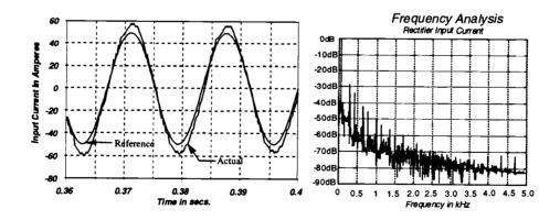
Figure 3.14 Time and frequency domain simulation result of rectifier input current with the proposed model based current controller under unity p.f. condition.  $f_{switch} = 5 \text{ kHz}, V_{grid} = 230 \text{ V} \text{ and } V_{dc} = 380 \text{ V}.$
