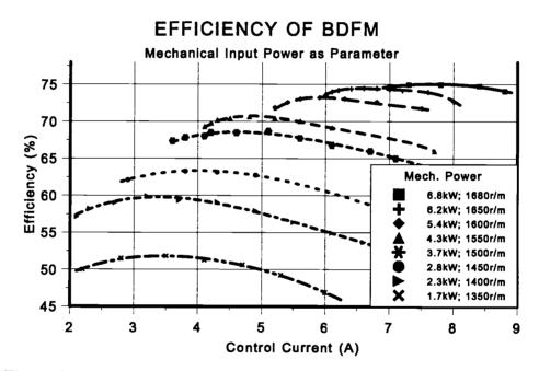
**Figure 2.6** Maximum efficiency point characterization of a 230 V, 7.5 kW prototype BDFM with input mechanical power as a parameter.
