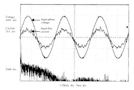
Figure 3.20 Rectifier operation with (-)21% line reactor inductance error.  $V_{ac} = 230 \text{ V}, V_{dc} = 390 \text{ V}, f_{switch} = 5 \text{ kHz}, \text{ load } \approx 6 \text{ kW}$
