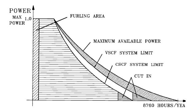
Figure 1.6 Power extraction from wind using VSCF and CSCF systems
