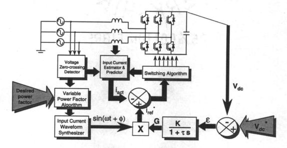
Figure 3.11 Sensorless version of the rectifier controller.
