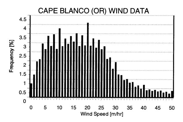
Figure 1.5 Sample annual wind speed distribution, illustrating the Rayleigh distribution of wind speeds.
