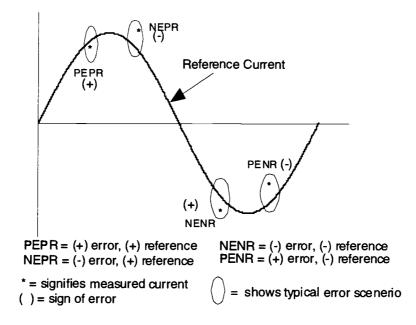
Figure 3.3 Possible current errors in each phase of the rectifier.
