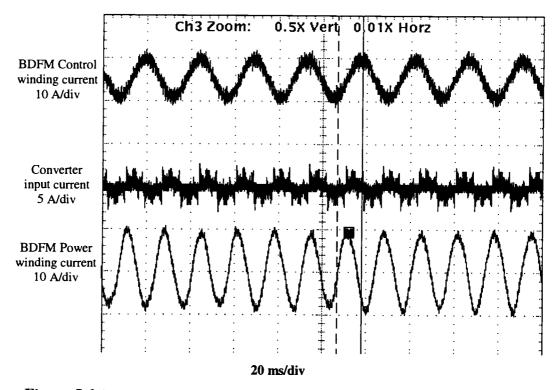
Figure 5.6 Representative current waveforms of the converter and the BDFM approximately at the maximum power point (P<sub>wt</sub> ≈ 1150 watts, shaft speed = 1525 r/min).
