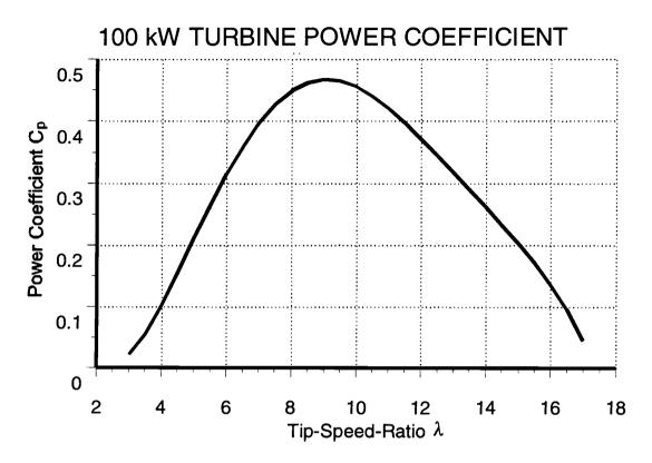
Figure 1.1 Power coefficient of a 100 kW wind turbine.
