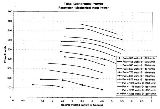
Figure 4.7 Variation of generated power with varying of control winding current for different input mechanical power.
