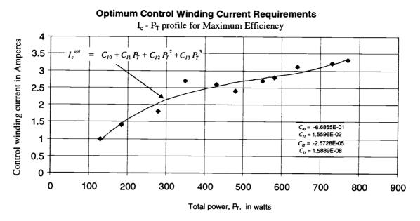
Figure 4.8 Optimum control winding current requirements for maximum efficiency operation of the prototype BDFM. The curve-fit polynomial, as shown, is the MEPT controller realization.
