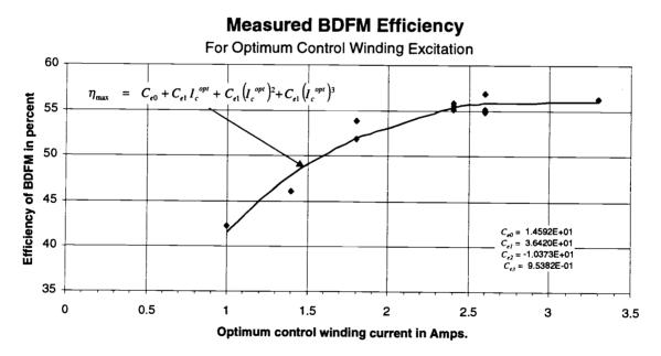
Figure 4.9  $\eta_{max} - I_c^{opt}$  profile of the prototype BDFM as implemented in the adaptive MPPT controller
