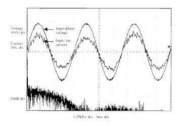
Figure 3.16 Unity power factor operation of the sensorless controller.  $V_{ac} = 230 \text{ V}, V_{dc} = 390 \text{ V}, f_{switch} = 5 \text{ kHz}, \text{ load } \approx 6 \text{ kW}$
