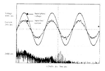
Figure 3.15 Experimental waveforms generated by the sensor-based controller.  $V_{ac} = 230 \text{ V}, V_{dc} = 390 \text{ V}, f_{switch} = 6.67 \text{ kHz}, \text{ load } \approx 6.5 \text{ kW}$
