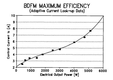
Figure 2.5 Optimal control winding current requirements to ensure maximum efficiency for a 7.5kW BDFM.
