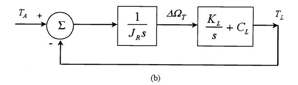
**Figure 1.4** Simplified wind turbine (a) mechanical model and (b) block diagram, typically utilized for determination of mechanical system resonances and responses
