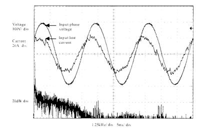
Figure 3.17 Leading power factor operation of the sensorless controller.  $V_{ac} = 230 \text{ V}, V_{dc} = 390 \text{ V}, f_{switch} = 5 \text{ kHz}, \text{ load } \approx 6 \text{ kW}$
