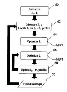
to determine the optimal control winding current setting, in 62.
