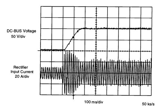
**Figure 3.6** Rectifier controller response to a 40% (280 V- 390V) step change in commanded dc-bus voltage. DC-bus capacitance =  $2400 \,\mu\text{F}$
