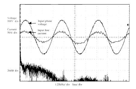
Figure 3.18 Rectifier operation with an (-)20% grid voltage error.  $V_{ac} = 184 \text{ V}, V_{dc} = 390 \text{ V}, f_{switch} = 5 \text{ kHz}, \text{ load } \approx 6 \text{ kW}$
