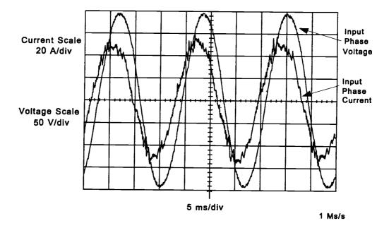
Figure 3.8 Leading 0.85 p.f. operation.  $V_{dc} = 390 \text{ V}$  $V_{ac} = 230 \text{ V}$ , load = 10 kW
