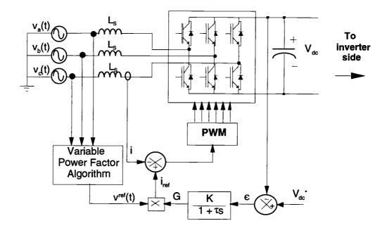
Figure 3.2 Sensor-based controller representation.
