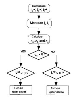
Figure 3.4 Switching logic of the rectifier.
