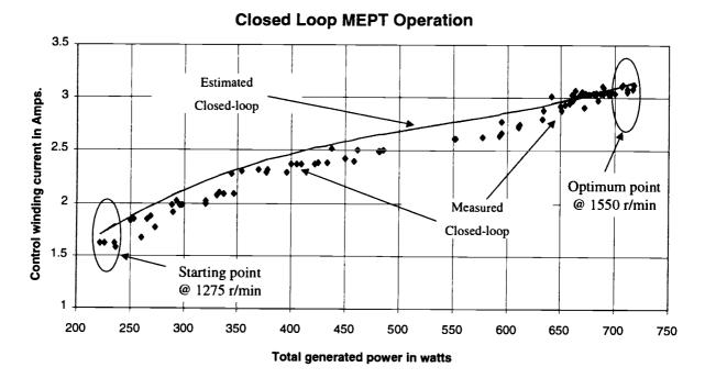
**Figure 5.4** Comparison of the measured and estimated control winding current for maintain optimum operation. The current has been estimated by substituting the measured power into the polynomial of Fig. 4.8.
