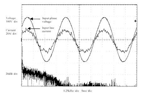
Figure 3.19 Rectifier operation with an imposed (+)17% grid voltage error.  $V_{ac} = 230 \text{ V}, V_{dc} = 390 \text{ V}, f_{switch} = 5 \text{ kHz}, \text{ load } \approx 5.5 \text{ kW}$
