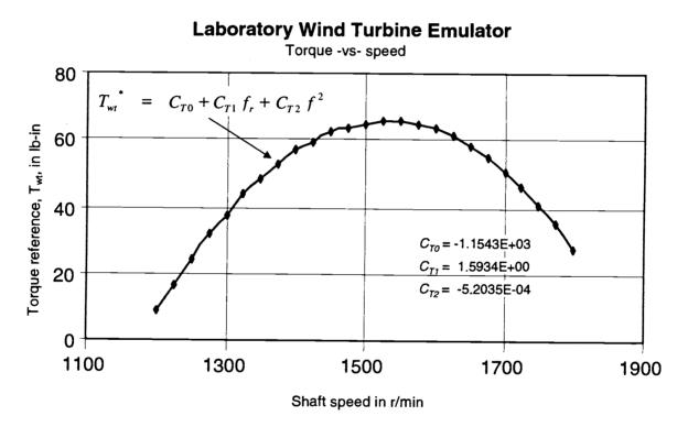
Figure 4.5 Desired torque-speed characteristic of the wind turbine emulator.
