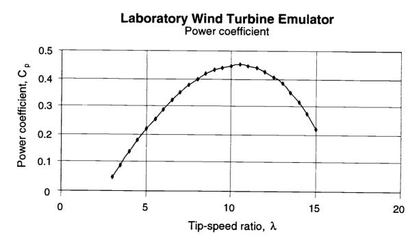
Figure 4.4 Power coefficient of the laboratory wind turbine emulator.
