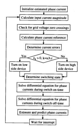
Figure 3.13 Simplified flowchart of the sensorless version of the rectifier controller
