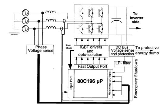
Figure 3.5 Sensor-based rectifier controller implementation
