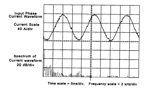
Figure 3.9 Leading 0.85 p.f. operation.  $V_{dc}$ = 450 V,  $V_{ac}$  = 230 V, load = 10 kW.
