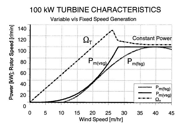
Figure 1.2 Variable and fixed speed power and speed characteristics of a 100 kW turbine.
