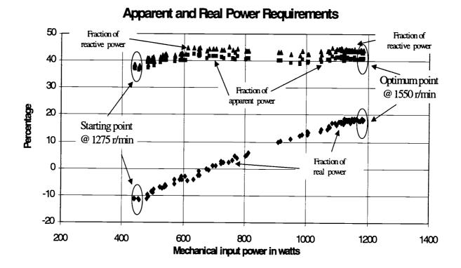
Figure 5.5 Power flow through the inverter as percentage of total apparent, real and reactive power.
