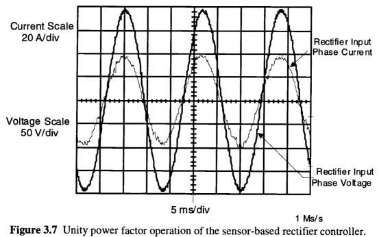
$V_{dc} = 390 \text{ V}, V_{ac} = 230 \text{ V}, \text{ load} = 10 \text{ kW}$
