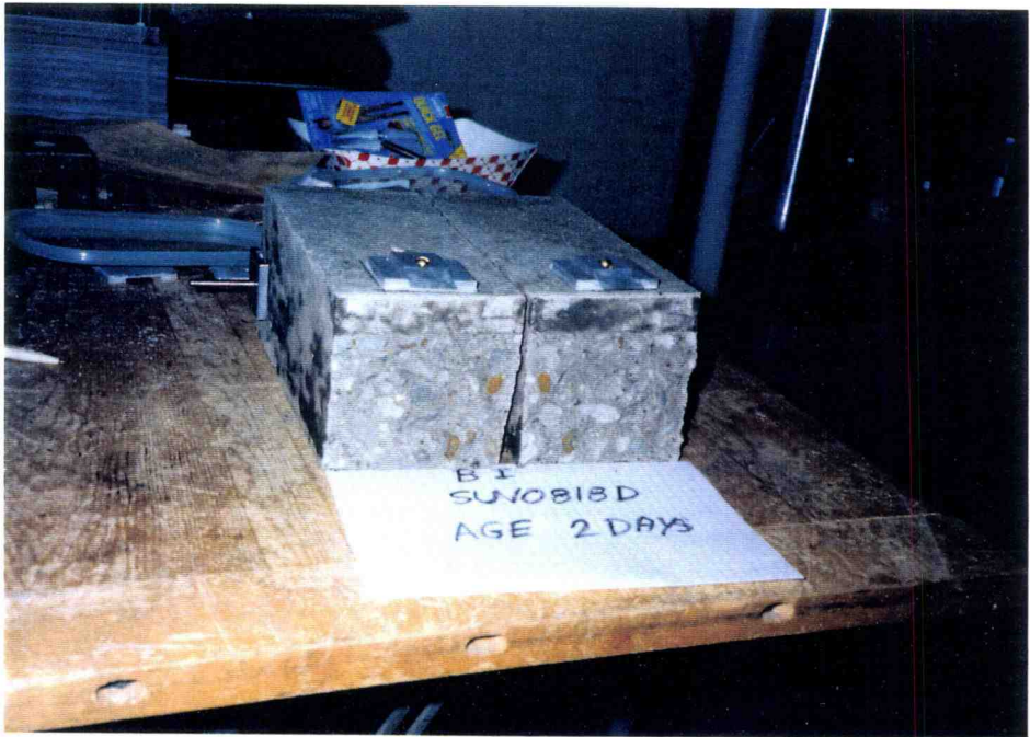
(b) bond failure and broken aggregates, 2 days
