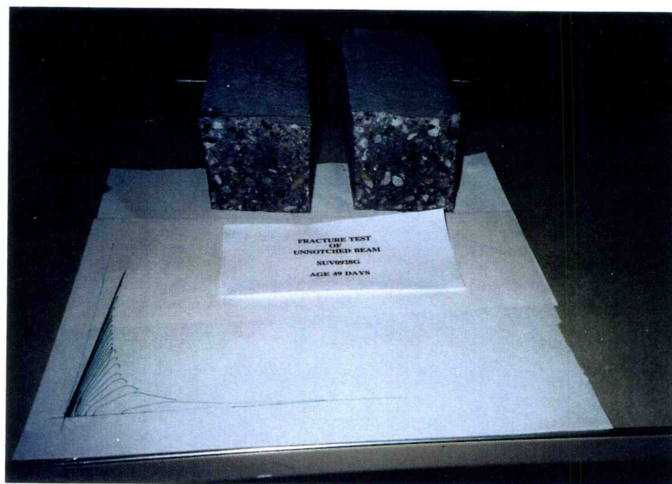
Figure 4.31 (continued) Difference failure mechanism at different ages (c) broken aggregates, 49 days
