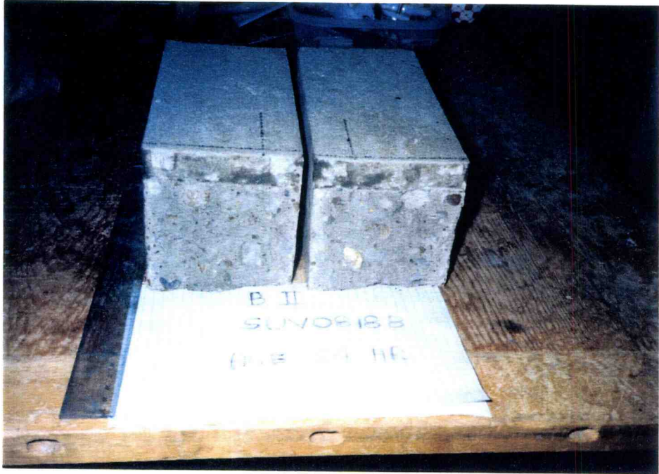
(a) bond failure, 24 hr
