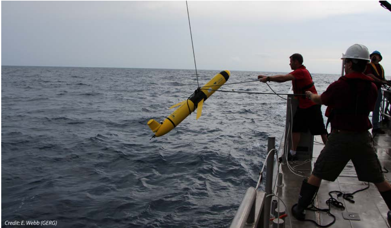
Figure 16.9. Pilot test of a profiling glider for hypoxia studies in the northern Gulf of Mexico by the Texas A&M University Geochemical and Environmental Research Group. Photo by Eddie Webb (Texas A&M University Geochemical and Environmental Research Group).
