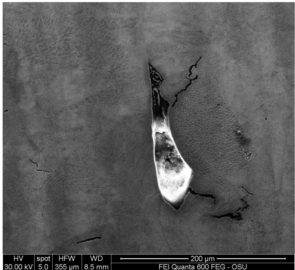
Figure 2.9: sample with low laser power showing LOF.
