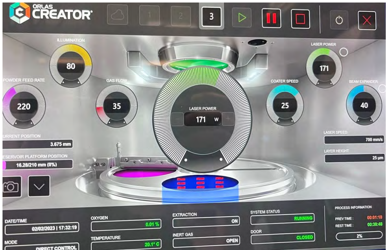
Figure 2.1 HMI screen of LPBF machine indicating oxygen level, temperature, inert gas, and extraction
