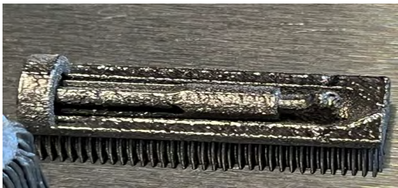
Figure 1.5: horizontal printing showing material distortion.
