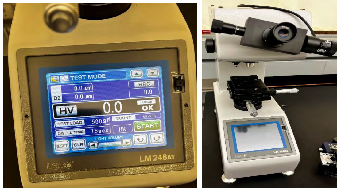
Figure 2.5: LECO LM248AT Micro-indentation Hardness Tester
