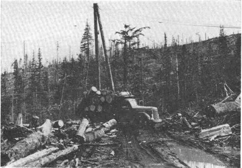
Figure 12. A-frame loader used for yarding small logs and for loading 8-foot wood. The A-frame and small donkey engine are mounted on the same sled.
