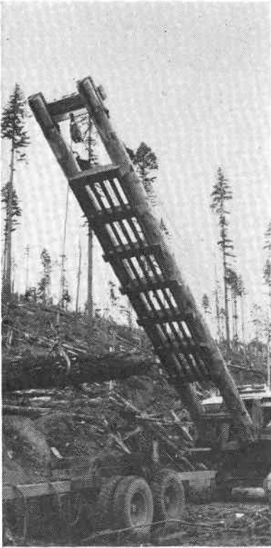
Figure 13. Heel-boom shovel loader used for loading medium-sized salvage logs.
