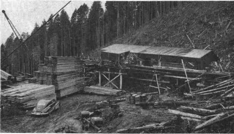
Figure 20. This 24-inch, sled-mounted, portable, log gang mill is moved into logged-over settings so that logs can be direct-yarded to the mill. Production is 14 to 15 thousand board feet per day with a 20-man woods and mill crew.
