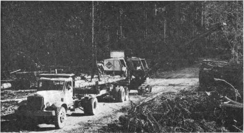
Figure 14. Small shovel with goose-neck heel boom used to load prelogged pulp species by Weyerhaeuser Timber Company.
