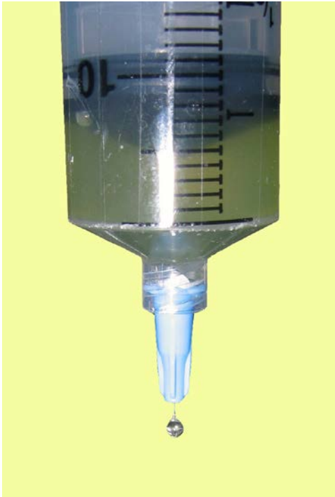
Figure 6. 40 ml Syringe with 22 gauge, modified needle dropping sodium alginate into calcium chloride.
