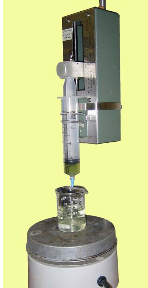
Figure 7. Syringe pump facilitating alginate extrusion into slow-mixing CaCl 2 .
