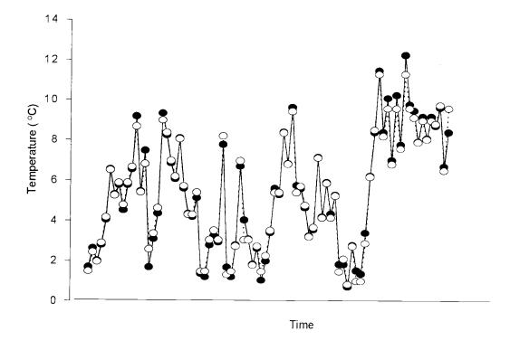
Figure 2.2. Temperatures (°C) over the course of the field exposure for a single mylar ( $\bullet$ ) and acetate (o) enclosure. Dots represent temperatures every 12 hours, starting at midnight of the first day. Statistical analysis for temperature was not performed on these data, but on means for the 4 acetate and 4 mylar enclosures taken at noon on five different days.
