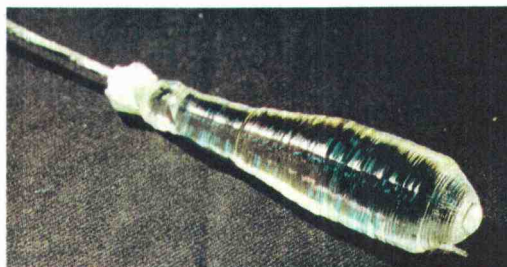
Figure 8.1. Boule of 15 at%-doped Yb:BOYS, grown on an iridium rod.
