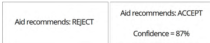
Figure 5. Sample cues for binary and graded automation. The binary aid on the left provides an absolute judgment, while the graded aid on the right communicates the strength of evidence assessed through a confidence rating.
