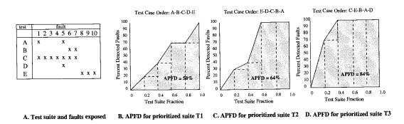
FIGURE 1.1: Examples illustrating the APFD metric.
