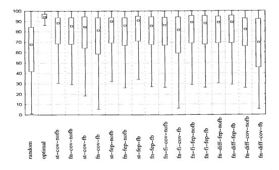
FIGURE 2.2: APFD boxplots for an "all programs" total. The horizontal axis lists techniques, and the vertical axes list APFD scores.
