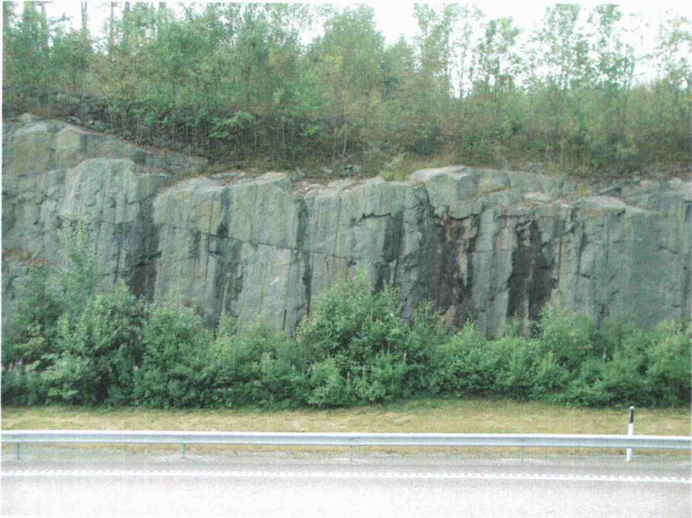
Figure 2-4. Photograph of a portion of the northern road cut, south side at Ekolsund showing exposure forming part of detailed mapping of Zone MY-1 (to right of center), in area which is wet due to groundwater seepage running down face of exposure (apparently mainly from one of the subhorizontal joints). The pattern of joints visible in this photo is typical of the area, outside of zones of more intense fracturing such as Zone MY-1. View is southward, prior to clearing brush for detailed mapping. Note guard rail in foreground for sense of scale. Photo by Sven A. Tirén.
