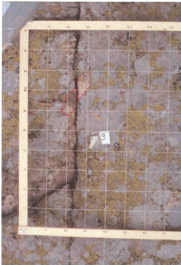
Figure 4-14. Detailed photograph from Äspö mapping area showing apparent left-lateral separation of about 3 cm of two fragments of an oblong, leucocratic inclusion which is cut by one of the main en échelon segments. The inclusion fragments are outlined by red dashed lines. The spacing between strings on the grid is 10 cm. North is upward in the photo, parallel to the reference line which passes through the 40 cm marks on the frame. The branching fracture which bifurcates from the main segment in the lower left corner, dips at low angle toward the SE. Note the point of bifurcation is from a bend in the main segment (interpreted as a compressional bend) from which fragmented material has apparently been weathered and eroded away.
