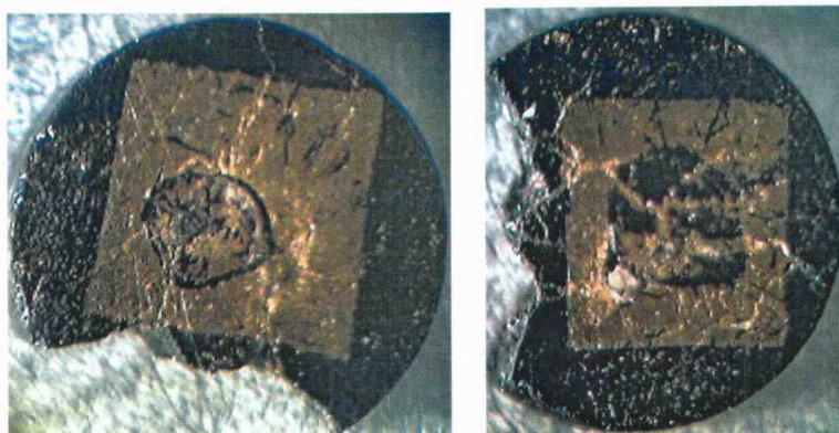
Figure 4.2 Images of two sides of the CCTO crystal grown by S. Wakimoto and obtained from A.P. Ramirez. The disc is 3.90 mm in diameter and 0.77 mm thick.
