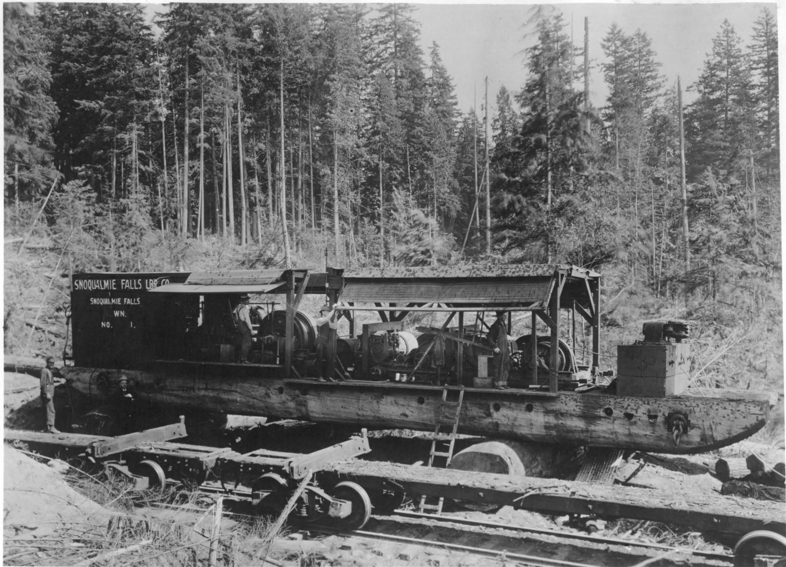
331195 ELECTRIC YARDER AND DUPLEX LOADER MOUNTED ON SLED USING HITC-5015-200HP- 600RPM- 3 PHASE- 60 CYCLE- 550 VOLT MOTOR WITH SOLENOID BRAKE AND SEMI MAGNETIC CONTROL ON YARDER AND 2 HITC-5013-A-75HP- 600RPM- 3 PHASE- 60 CYCLE- 550 VOLT MOTORS WITH CR9510 BRAKE AND SOLENOID LOAD BRAKE ON LOADER INSTALLED AT SNOQUALMIE FALLS LUMBER COMPANY, SNOQUALMIE FALLS, WASHINGTON.
