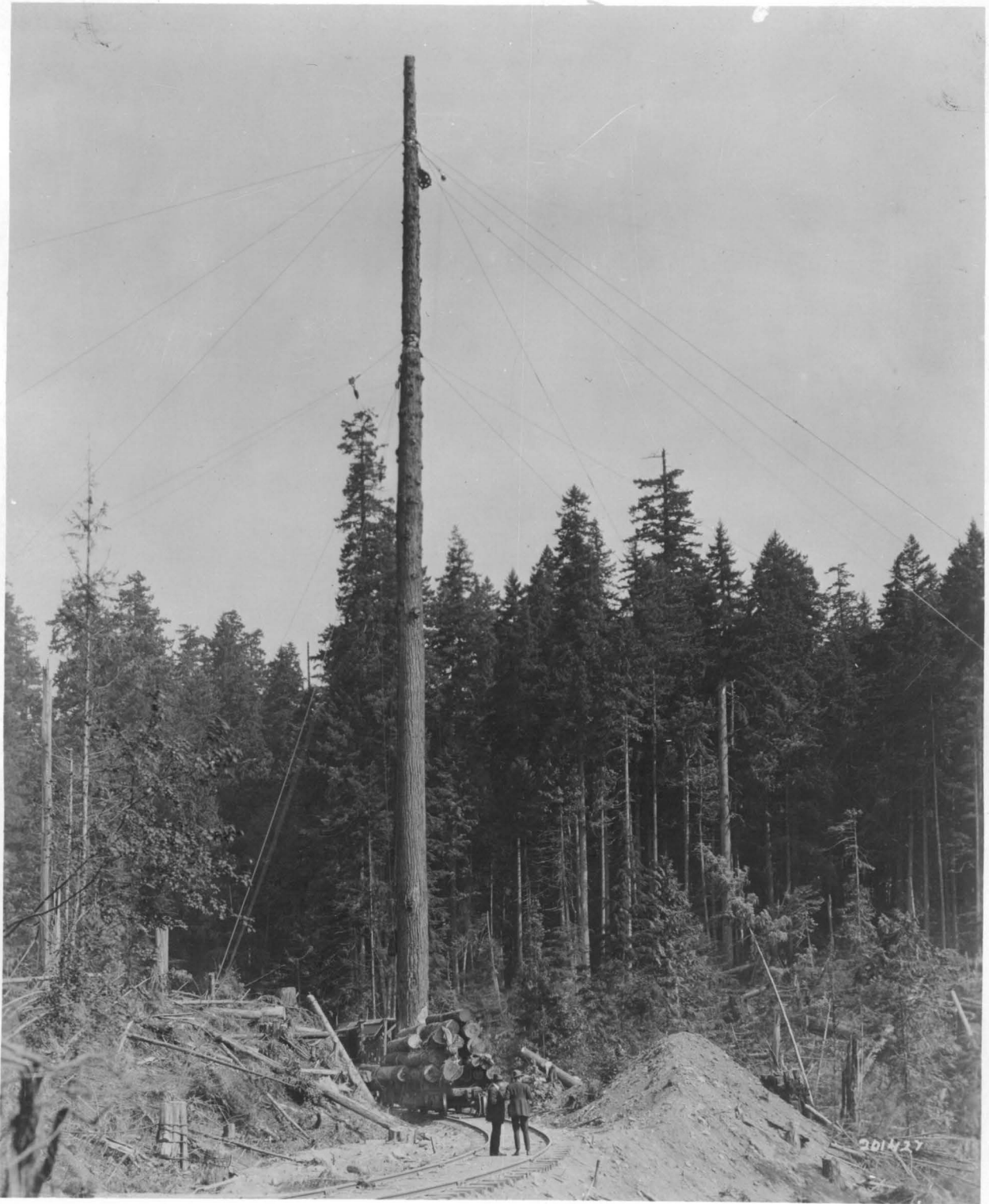
331194 SPAR TREE AND RIGGING FOR ELECTRIC LOGGING OPERATIONS. SNOQUALMIE FALLS LUMBER COMPANY, SNOQUALMIE FALLS, WASHINGTON.
