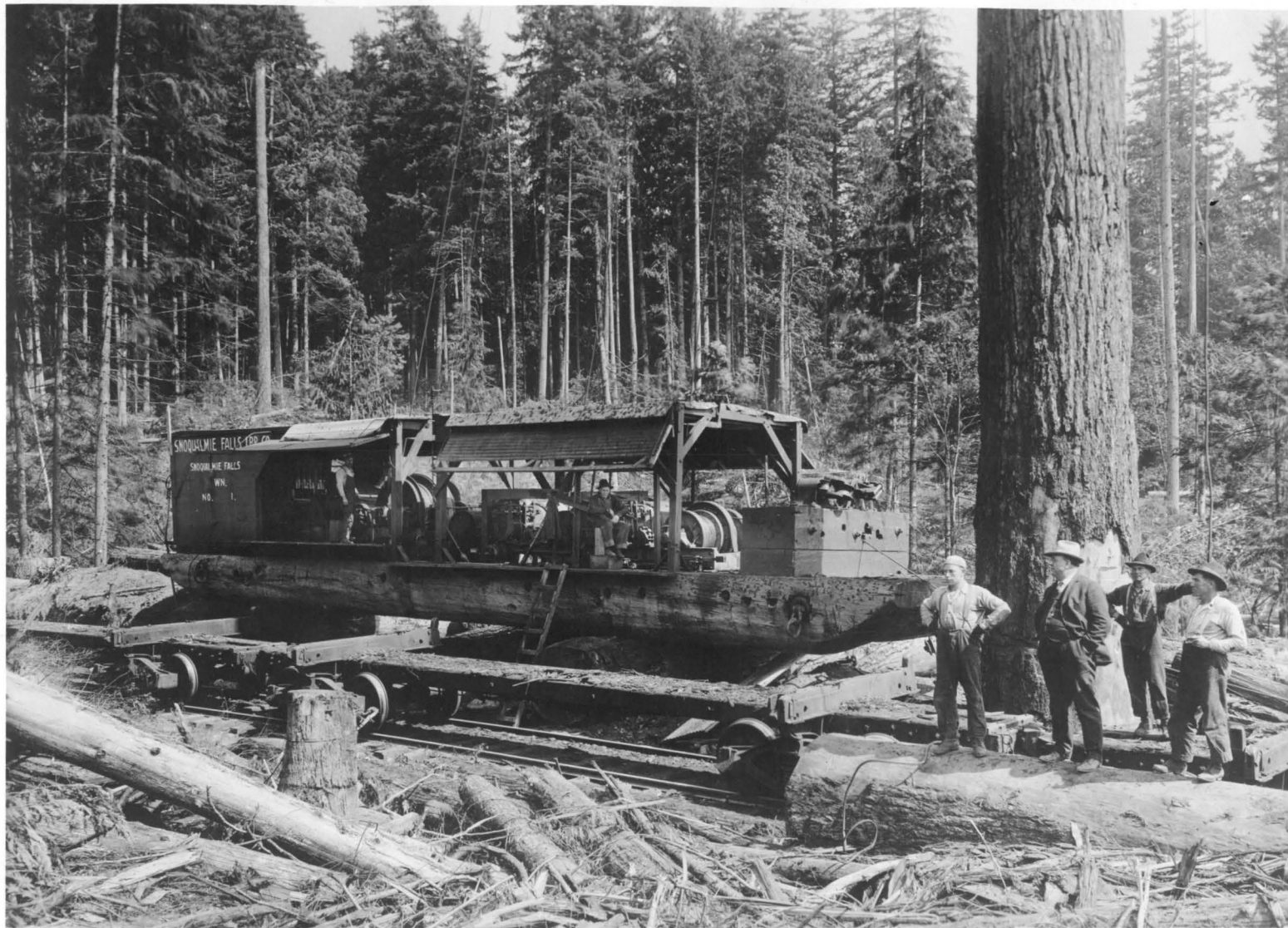
331197 ELECTRIC YARDER AND DUPLEX LOADER MOUNTED ON SLED USING HITC-5015-200HP- 600RPM- 3 PHASE- 60 CYCLE- 550 VOLT MOTOR WITH SOLENOID BRAKE AND SEMI MAGNETIC CONTROL ON YARDER AND 2 HITC-5013-A-75HP- 600RPM- 3 PHASE- 60 CYCLE- 550 VOLT MOTORS WITH CR9510 BRAKE AND SOLENOID LOAD BRAKE ON LOADER INSTALLED AT SNOQUALMIE FALLS LUMBER COMPANY, SNOQUALMIE FALLS, WASHINGTON.
