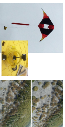
Figure 1. Kite data collection system and an example set of two overlapping images acquired with this system
