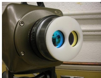
Figure 4: Stereoscopic Lens and camera with filter attachment. On the right is the bandpass filter and on the left is the high pass filter
