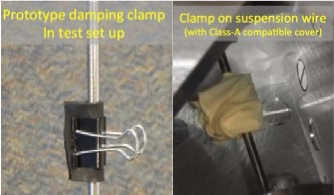
Figure 2.3: The setup of the prototype damping clips on the flexure.
