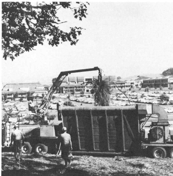
The Camran Air Curtain Combustor is one answer to smokeless burning adjacent to population centers. --Photo taken at a recent demonstration at Lane Community College, Eugene.
