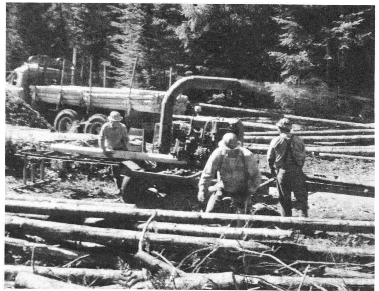
Portable post peelers utilize thinnings either in the woods or at a peeling yard.
