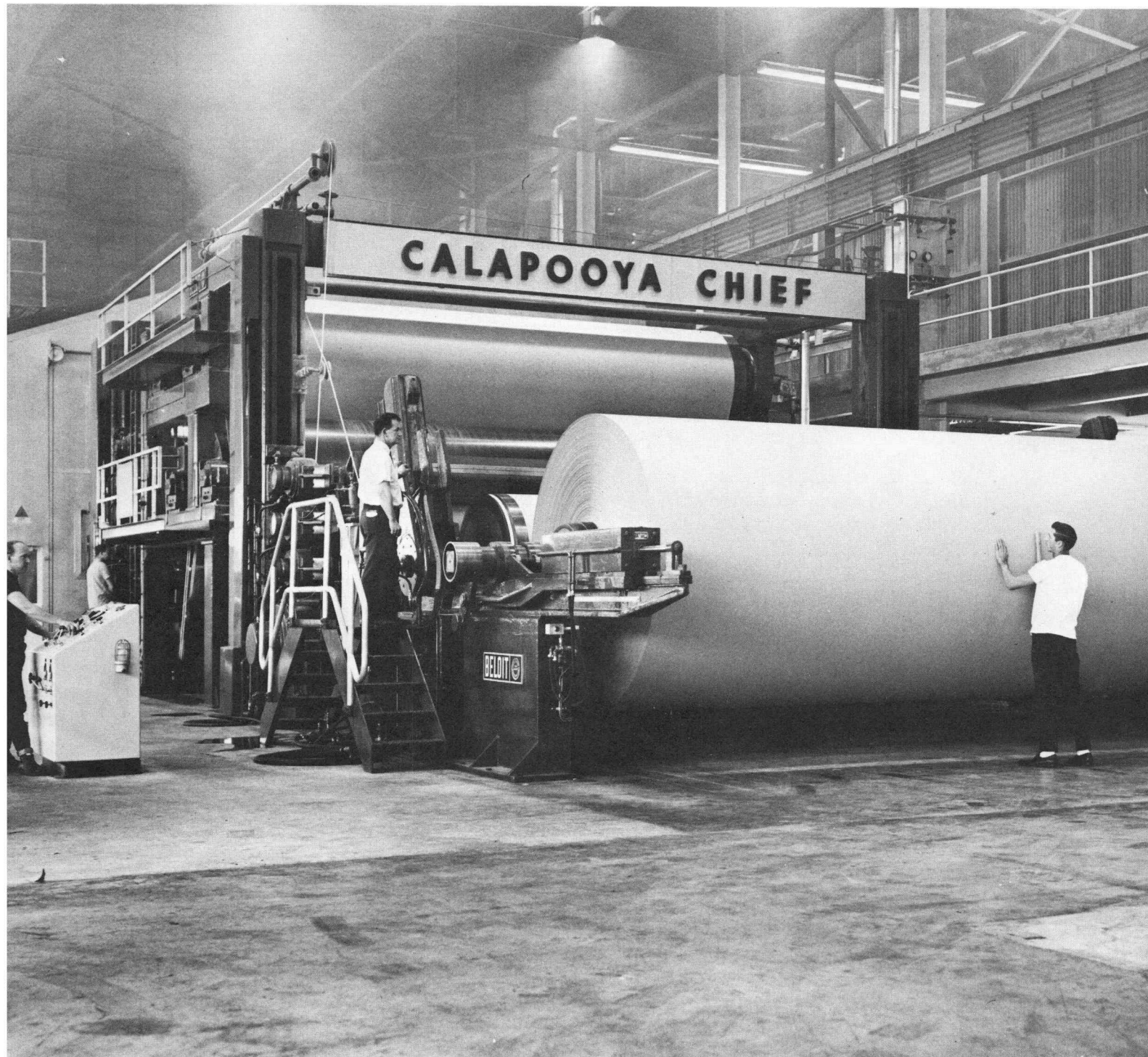
The "Calapooya Chief" produces an average of 750 tons or 400 miles of Kraft paper per twenty-four hour period. (Photo by Weyerhaeuser Co.)
