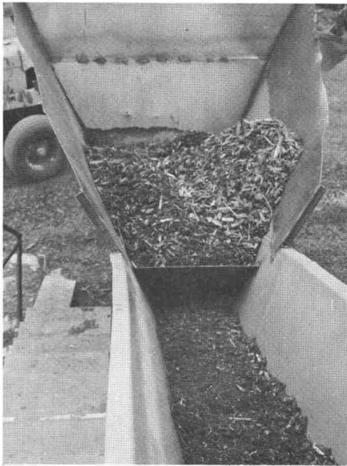
Figure 30. Fuel feed hopper and conveyor for the test burner.
