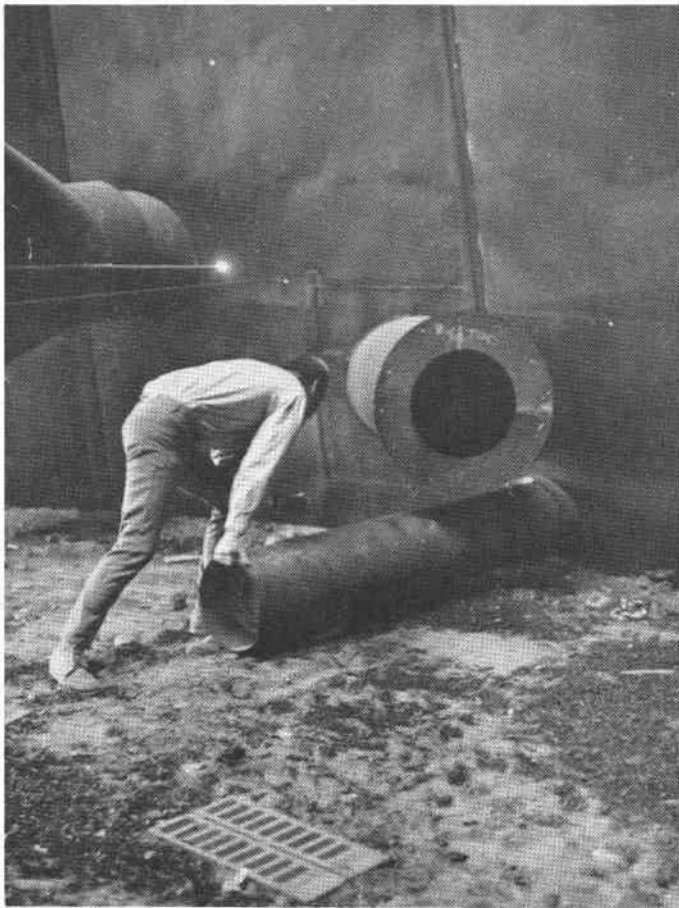
Figure 22. Recirculation intake (above) and movable gas burner (below) on the test burner.
