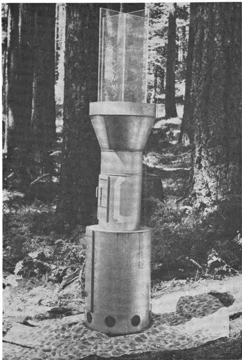
Figure 1. Metal olfactometer used for selective sampling and field testing of volatile materials.
