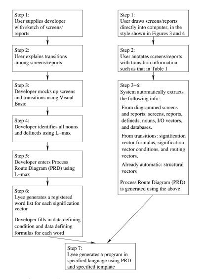
Fig. 5. A strategy (right side) for applying end-user programming to the current (left side) Lyee methodology (also assumes incorporation of work by other collaborators in relevant ways).
