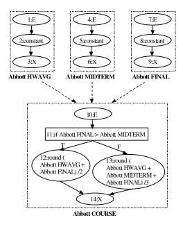
Fig. 2. A partial cell relation graph of Figure 1. These are the formula graphs for the top row ("Abbott, Mike"). Dashed arrows indicate dataflow edges between cells' formula nodes. For clarity in this figure, we preface cell names with "Abbott" instead of with the internal IDs actually used.
