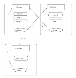
Fig. 4. An example screen transition diagram.
