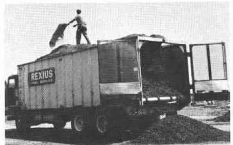
Figure 10. Hogg fuel being discharged from a self-unloading truck.
