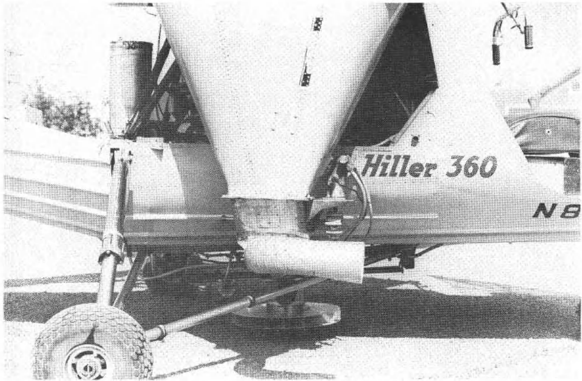
Plate VII. Bait and Seed Disseminating Mechanism, Side View
