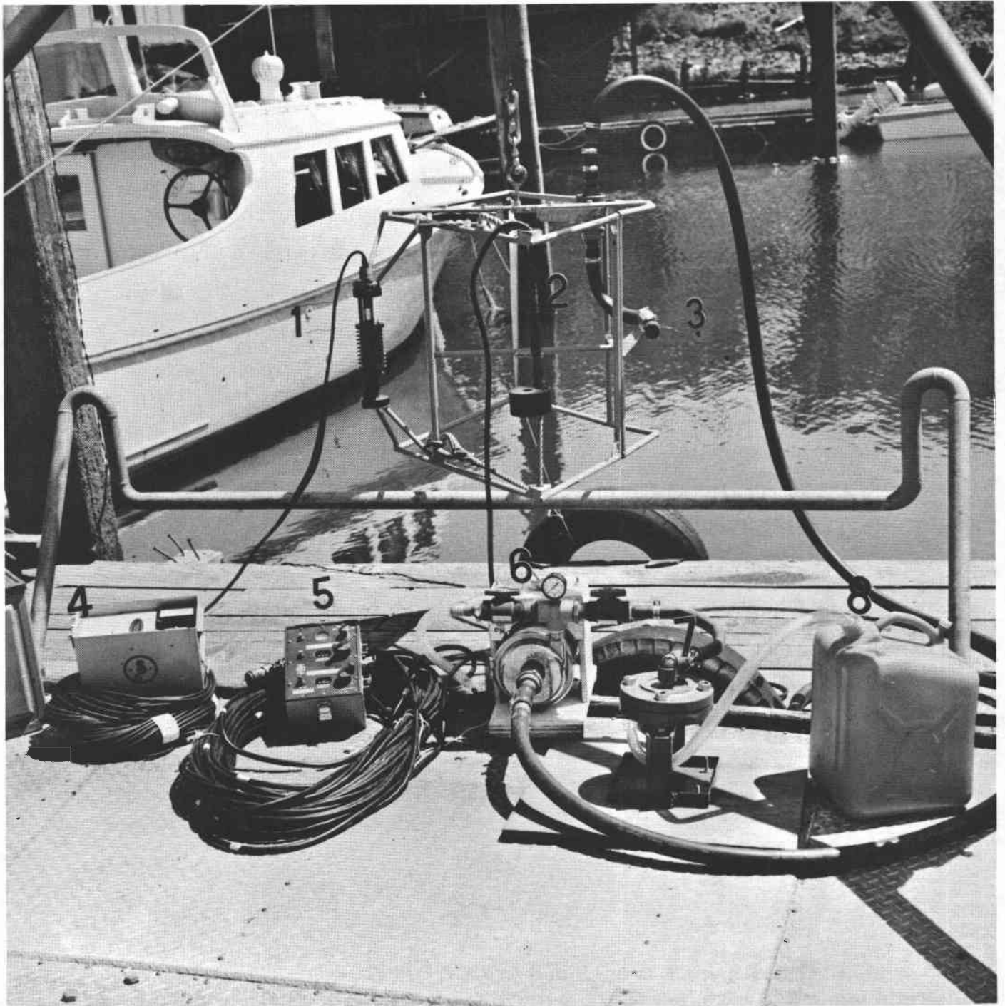
Figure 1. Instrument package ready for sampling: (1) Transmissometer underwater sensor; (2) Conductance-Temperature cell; (3) water intake for pumping; (4) Transmissometer unit; (5) Conductance-Temperature unit; (6) stainless steel pump; (7) filter unit; (8) polyethylene storage container.
