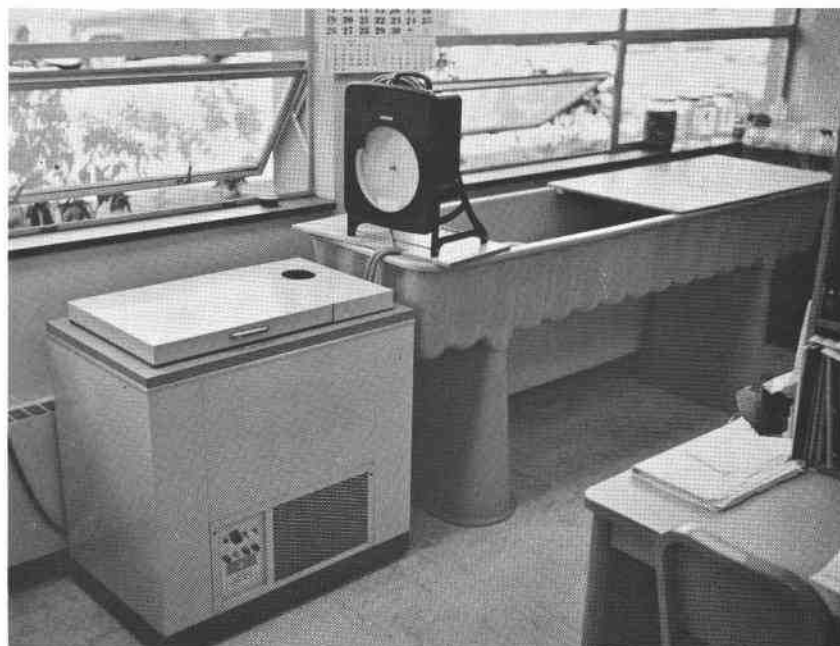
Figure 2. A refrigeration unit, fish trough, and temperature recorder which will be used to study radionuclide metabolism in marine organisms.
