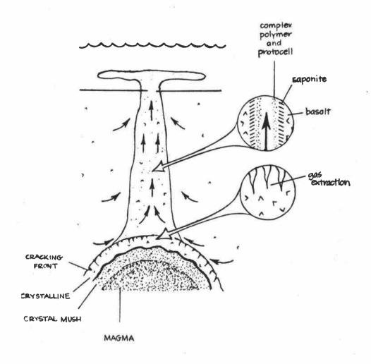
Figure 2a. Model seawater hydrothermal system.
