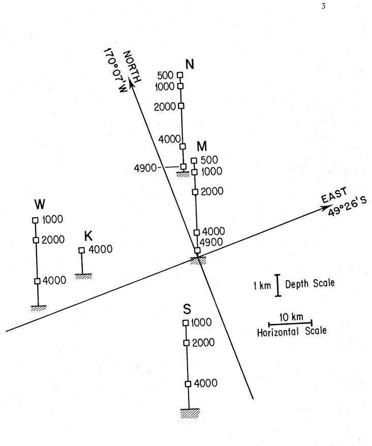
Figure 2. Positions of current meters deployed in the cluster array near  $49^{\circ}30$ 'S, 170°W from April to November 1978.
