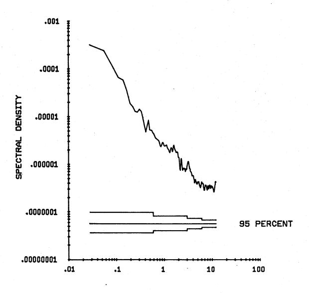
UNFILTERED PRESSURE, 2013 METERS AT NGAIO.
