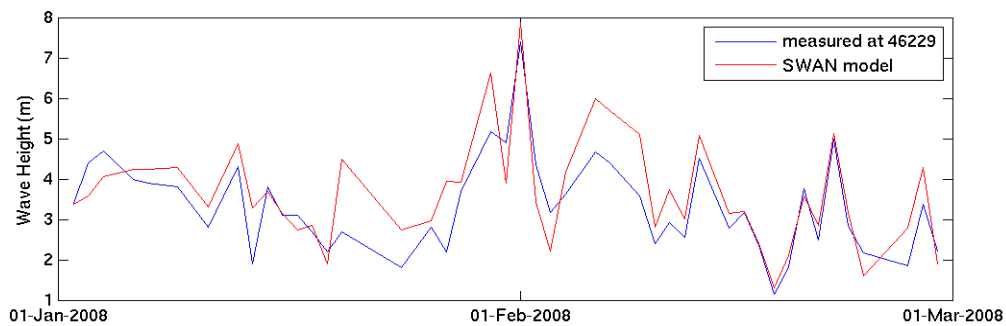
Figure 4: Comparison between predicted (red) and observed (blue) wave height at NDBC buoy 46229 over 2 months of simulations.
