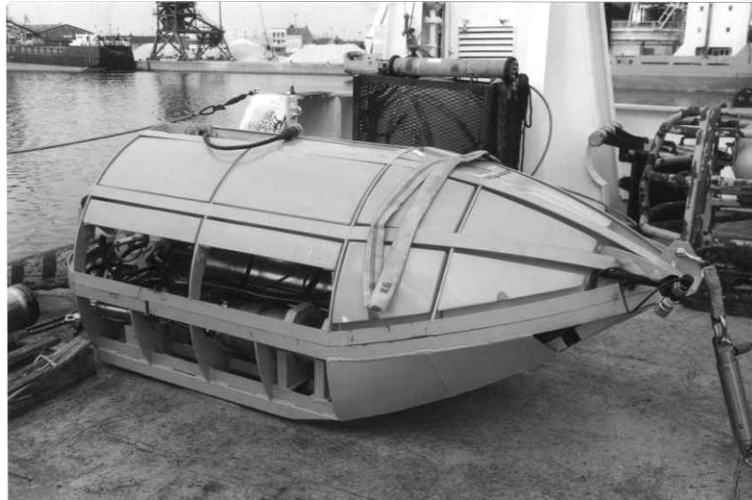
GAMBAS® refraction seismic system – seabed tow sled
