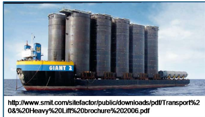
Figure 67 Smit Marine Semi-submersible Barge
