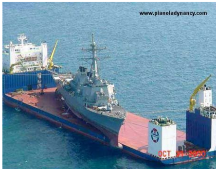
Figure 66 Semi-submersible Barge with USS Cole
