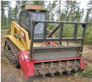
Figure 52. Machines equipped with (A) cutting blades and (B) grinding teeth are used to reduce understory trees and shrubs in some forest types to lower fuel loads.
