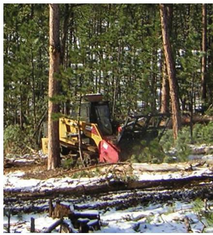
*Figure 53. A grinder mulching understory trees and shrubs in a pine forest to reduce fuel loads and continuity.*
