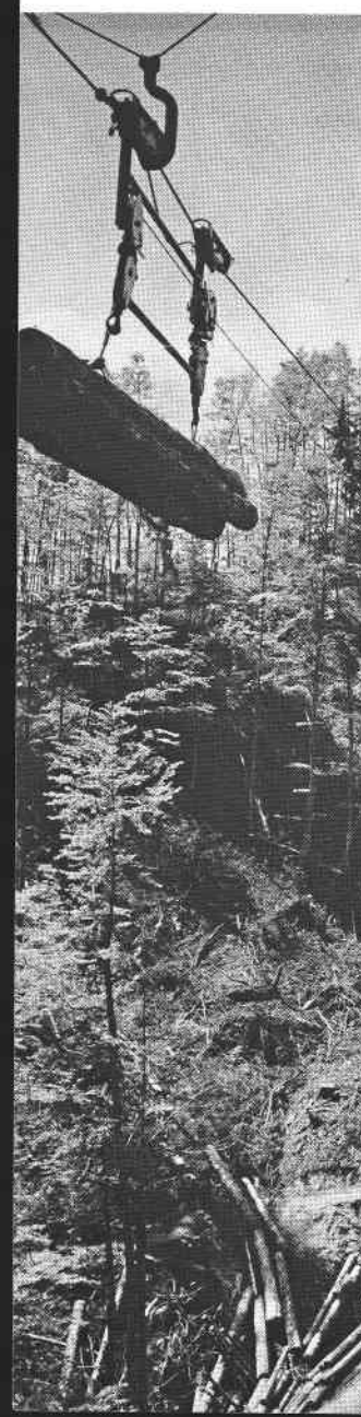
Below left: Cable logging with the "Huber" system. (Photos by G. Meister.)
