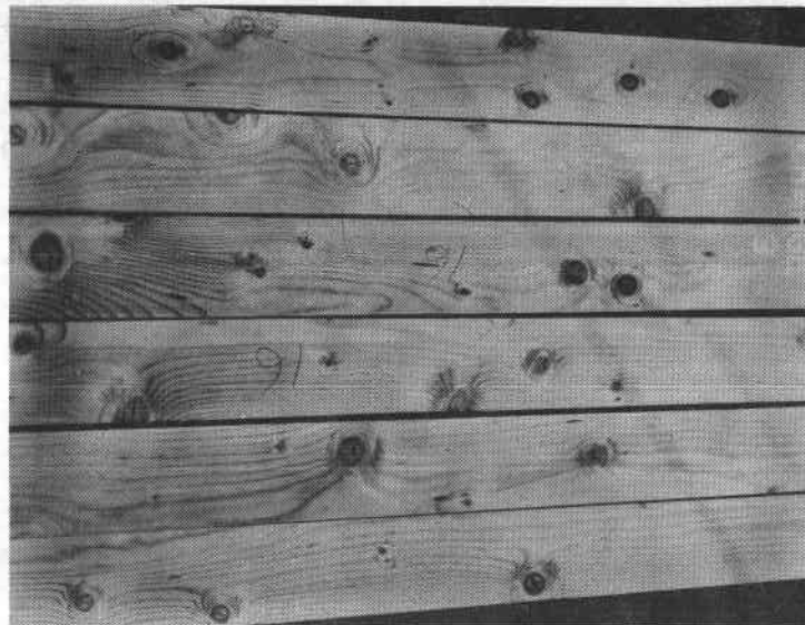
FIGURE 22. CONDITION OF KNOTS AFTER SURFACING: CHARGE 9.
