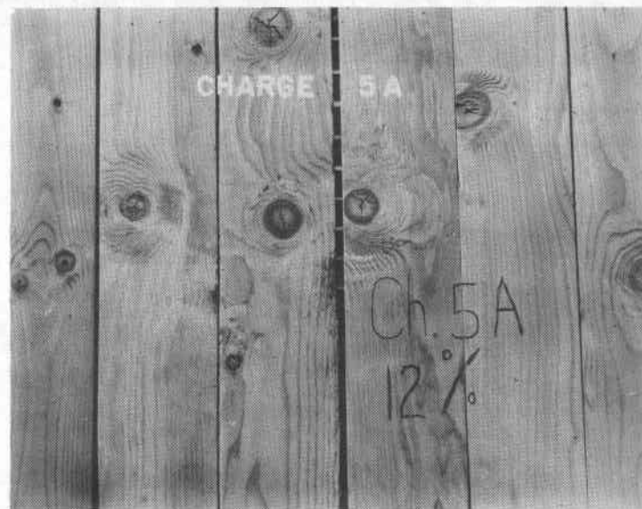
FIGURE 18. CONDITION OF KNOTS AFTER SURFACING: CHARGE 5A.
