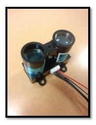
Figure 3.1.3: Lidar Lite V2
