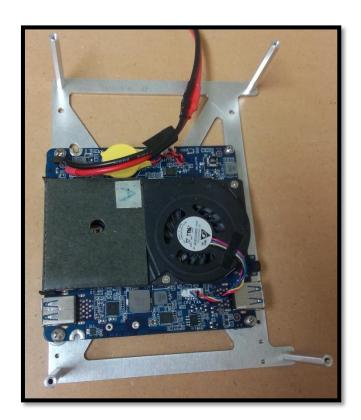
Figure 4.2.4: Bottom Plate with Brix CPU and Standoffs attached
