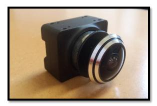
Figure 3.1.2: Chameleon3 camera with fish-eye lens
