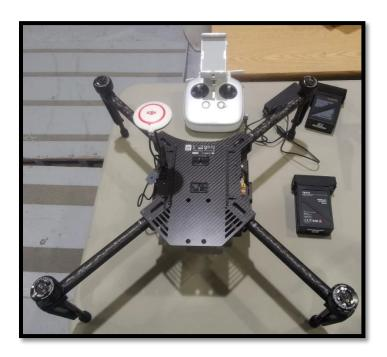
Figure 1.2: A stock DJI Matrice 100 with controller and TB47D Battery
