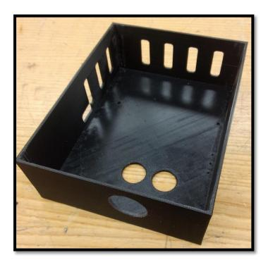
Figure 4.2.2: 3D Printed Bottom Shell Piece
