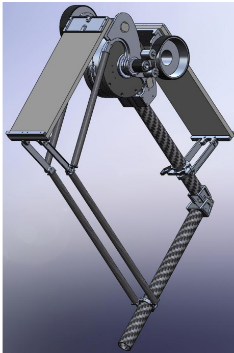
Figure 7.2: Current ATRIAS design. Rendering of monopod with two force-controlled joints and series compliance.
