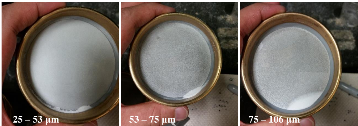
Figure 15: Distribution of particle sizes for a sample of strontium oxide that has been stored for one month after heat treatment and initially being sieved to 53 – 75 \mu\text{m} . Distribution of new particle sizes are from 25 – 53, 53 – 75, and 75 – 106 \mu\text{m} .
