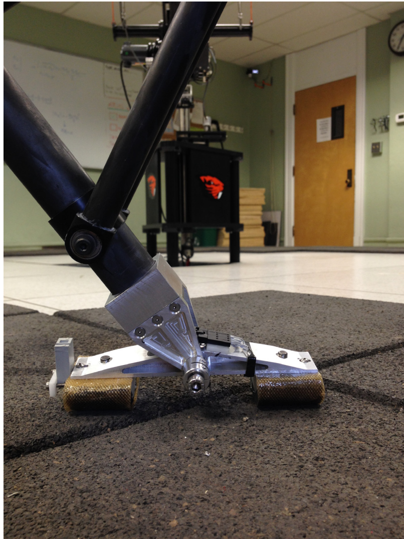
Figure 16: Foot mounted to ATRIAS.
