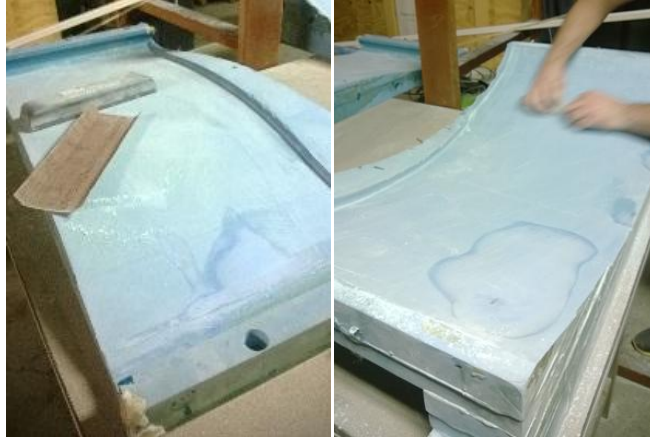
Figure 166: Re-sanding surfaces to remove excess epoxy resin
