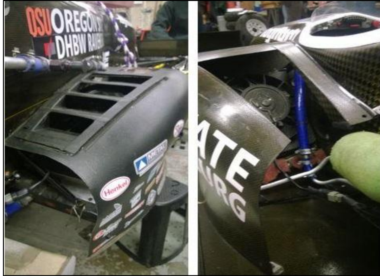
Figure 36: 2012(left) and 2013(right) Side-Pods illustrating difference between lower removal and exit area.
