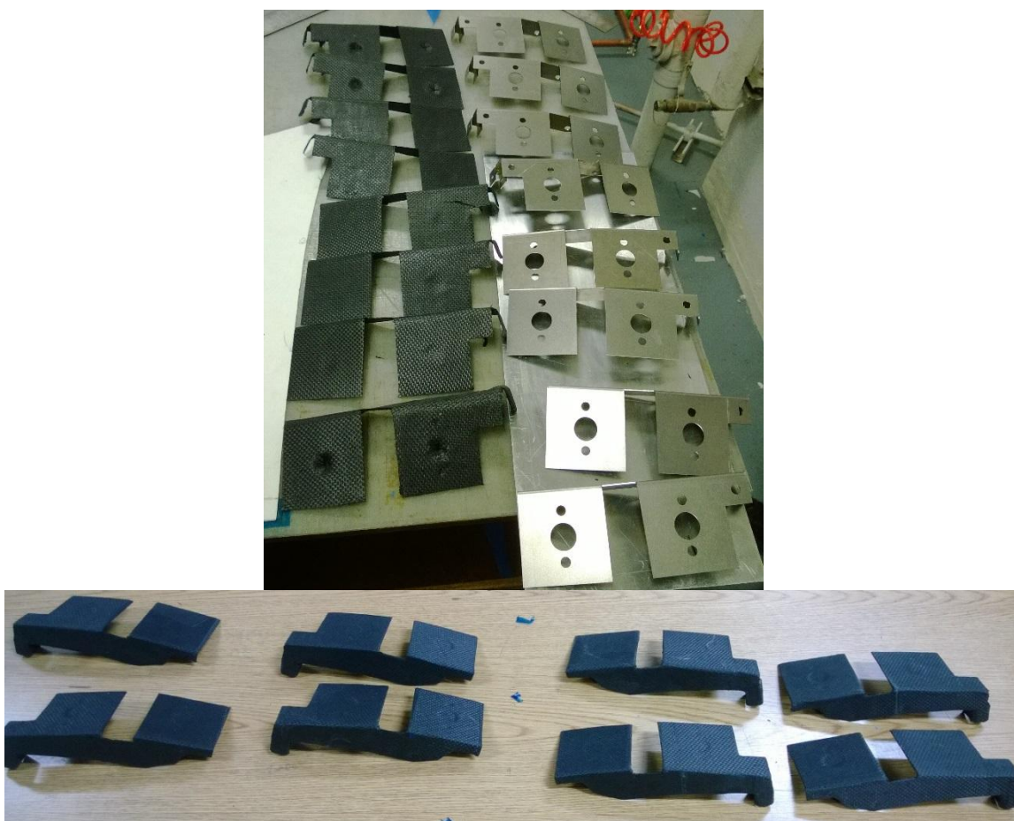
Figure 213: One oven cure cycle batch of eight finished brackets
