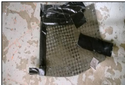
Figure 32: Radiator Carbon-Fiber Ducting with Gorilla Tape
