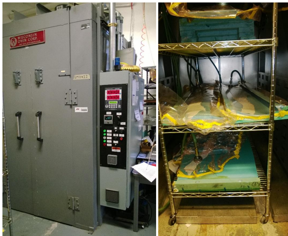
Figure 191: Oven curing of RenShape molds
