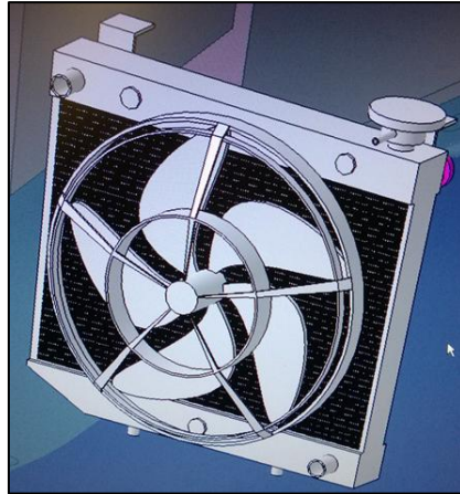
Figure 116: Original fan-radiator package in CATIA V5
