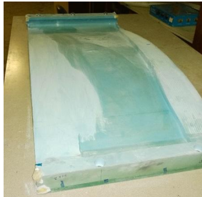
Figure 163: Mold removal with initial 40-grit roughing operation
