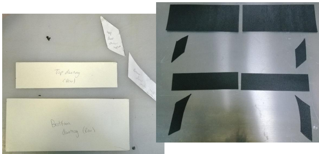
Figure 216: Rear ducting templates (left) and cured components (right)
