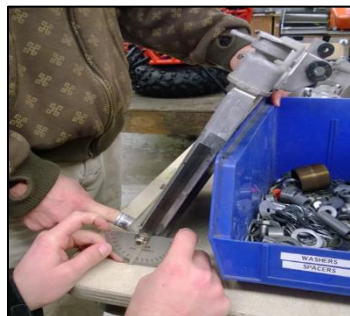
Figure 57: Radiator water fill and air bubble check at desired mounting angle.
