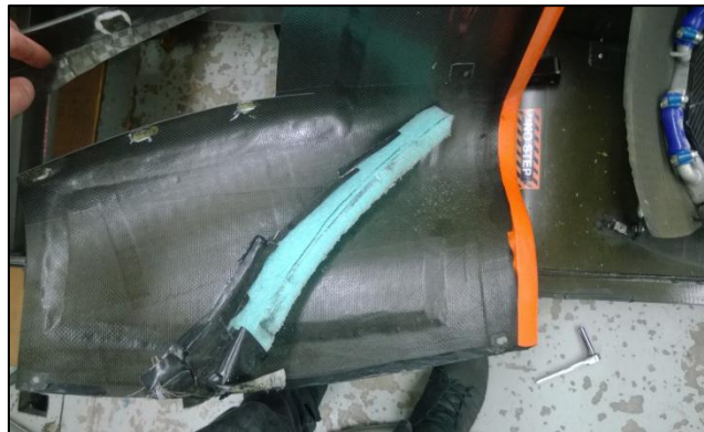
Figure 33: Driver side, side-pod with post-processing manufacturing additions using foam and tape to further seal and direct the air towards radiators.
