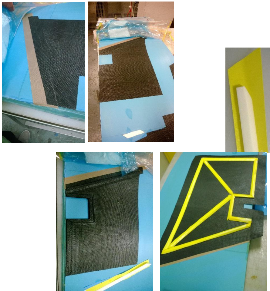
Figure 195: Side-pod lay-up process
