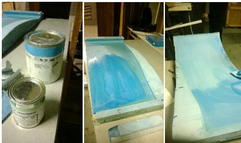
Figure 165: Filling low areas with Ren-Weld epoxy resin
