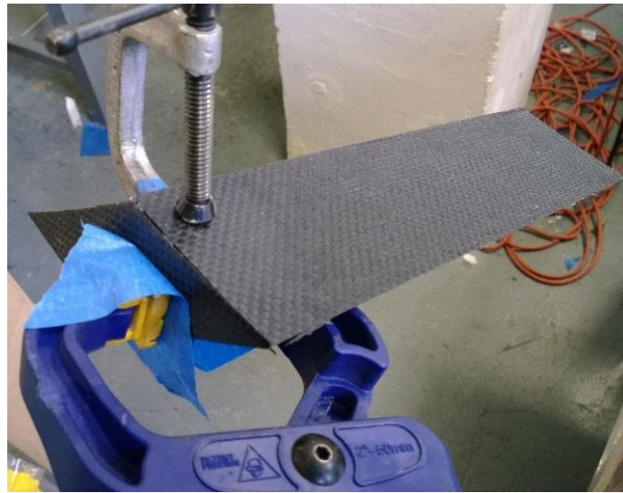
Figure 217: Epoxy process of assembling rear ducting components
