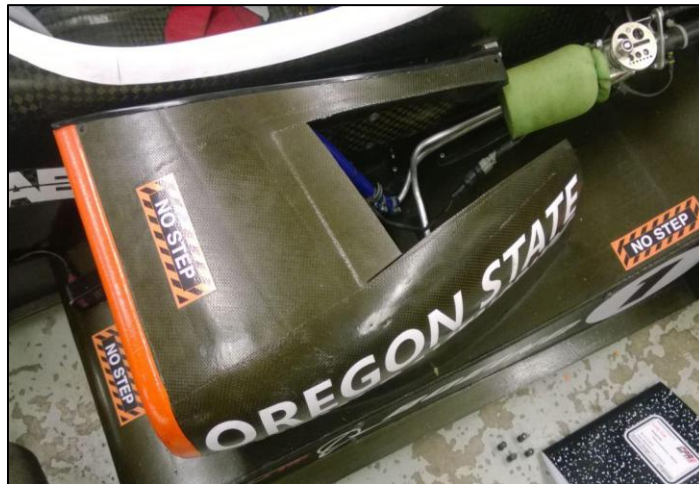
Figure 27:2013 Side-Pod with Louvers Removed
