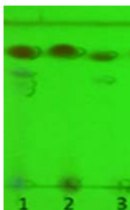
Figure 3.11. TLC Analysis of MBRL 251 extracts [CHCl 3 -MeOH (10:1)]. 1, EtOAc extract; 2, BuOH extract; and 3, cell-cake extract.
