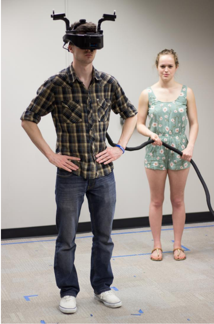
Figure 2. The Sensics zSight HMD worn by participants for immersive conditions, along with the infrared trackers mounted on the HMD. These gave its position and orientation, allowing the wearer to move around the virtual lab model as they moved around the actual tracking space. A researcher followed behind the participant, managing the cable and ensuring safety.
