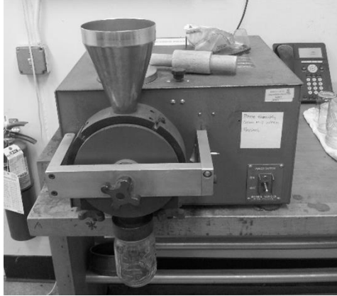
Figure 3.2 -Coarse (particle size) mill used to grind feedstocks at EPA
