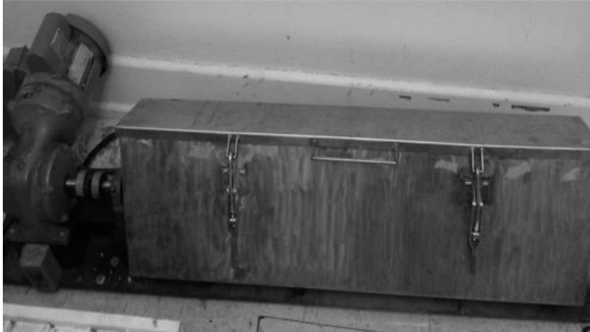
Figure 3.6- The tumbler used for the batch kinetics and isotherm tests is stored in Merryfield Hall.
