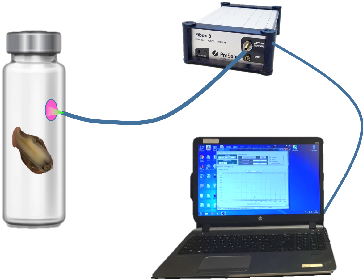
Figure 3-1 Experimental set up for measuring individual respiration rates of juvenile red abalone. Individuals were placed in sealed ground glass vials with an oxygen sensitive optode. A Fibox 3 Oxygen Sensor by PreSens was used to measure the in situ concentration of oxygen at the beginning and end of the assay in order to calculate rate of oxygen usage. Between measurements, vials were stored in a 10 °C water bath.
