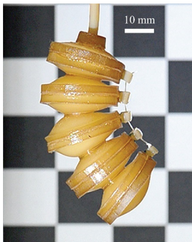
Figure 1. PGS-CaCO 3 assembled into pneumatic actuators by laser cutting and adhering layers together.
