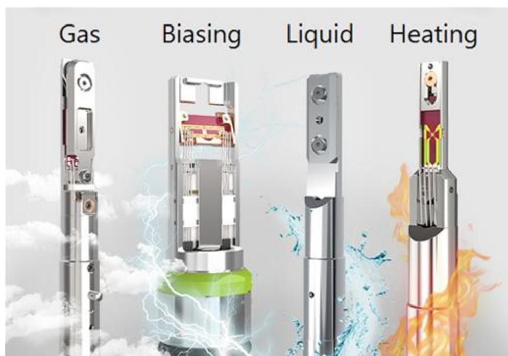
Figure 4.1. A sample of different TEM holders which allow for different in-situ experiments. From left to right: A holder allowing gas flow onto the sample, a holder allowing voltage biasing of the sample, a holder allowing viewing of liquids, and a holder allowing sample heating 1 .
