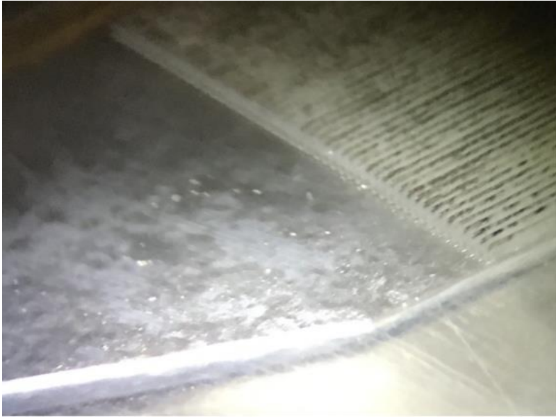
Figure B.8. Magnified view of a high aspect ratio polycarbonate lamina showing the deeper header and the uniformly tall fins that form the channels. The channels are 250 \mu\text{m} wide and over 500 \mu\text{m} tall before they are polished flat. The fins that form the channel walls are \sim 100 \mu\text{m} wide at the middle and form nearly rectangular channels.
