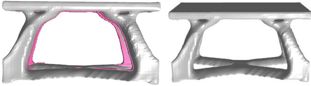
Figure 4.13: Unmanachable solid shown in pink over the as-designed part from a single piece (left) and using the optimal manufacturing plan (right)
