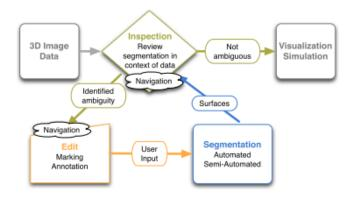
Figure 2.1: Integrated pipeline of segmentation, inspect, and edit.
