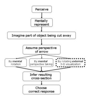
Figure 4.14: An informal model of the processes involved in performing the task of visualizing a cross-section [52].
