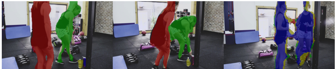
Figure 2.9: Sequence of frames showing the instance region-growing problem: each segment instance grows to encompass all instances, leading to incorrect (and conflicting) instance IDs. However, all foreground objects are still covered.
