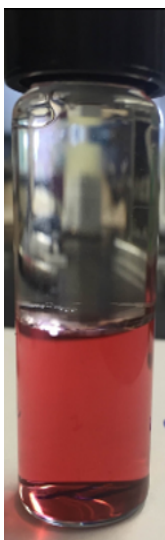
FIGURE B.1: The shake flask method for octanol water partitioning performed using Au NPs. Particles were visually observed to partition to the aqueous phase.
