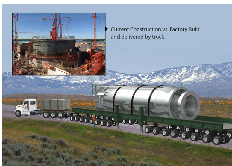
Figure 1.2: NuScale small modular reactor portability. Image from NuScale Power [5].
